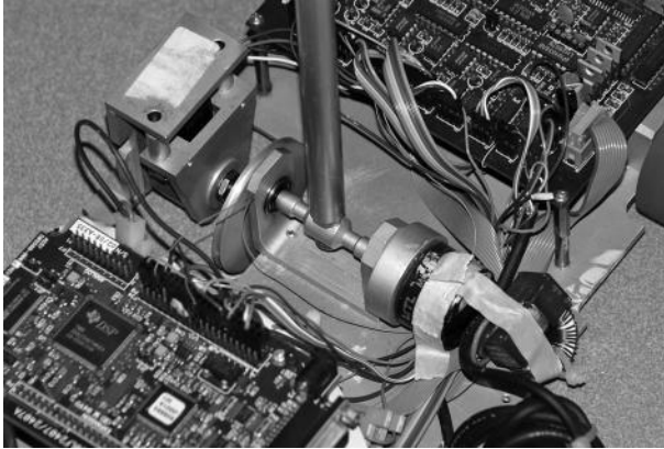
FIGURE 10.21 The drop-encoder and the pole support system.
