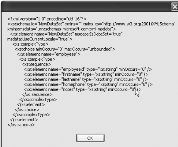
Figure 7-14. Schema extracted by using the ReadXmlSchema() method
