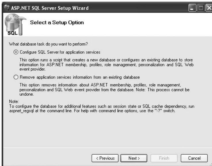
Figure 11-26. Step 2 of the aspnet_regsql.exe tool
