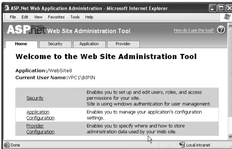
Figure 11-28. The Web Site Configuration tool
