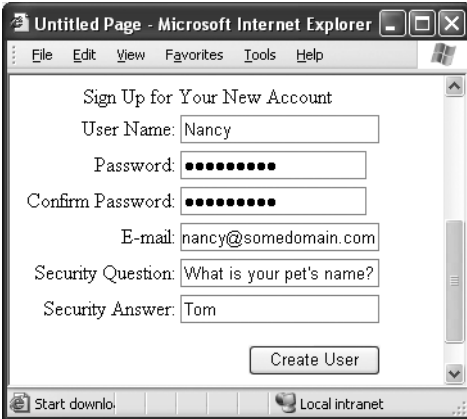
Figure 11-32. Creating new users by using the CreateUserWizard control
