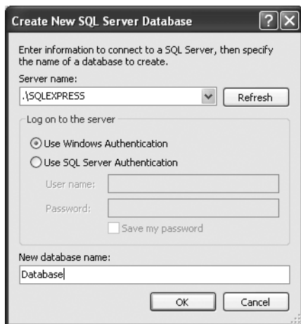
Figure B-1. Creating a new database by using Server Explorer
