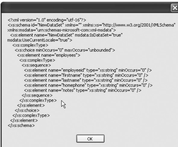
Figure 7-15. Schema extracted by using the InferXmlSchema() method
