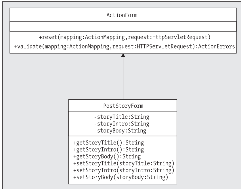
Figure 3-3. PostStoryForm's relationship to the ActionForm class
