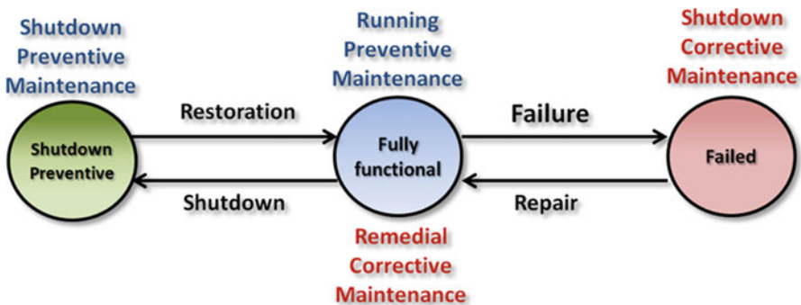
Fig. 2.13 Preventive and corrective maintenance on a three-state repairable system
