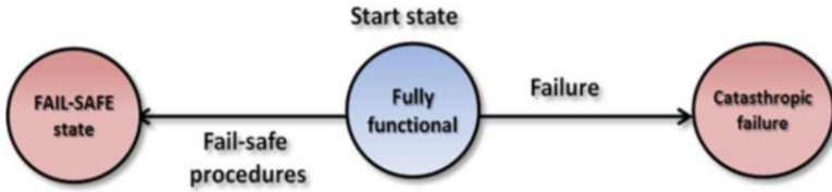
Fig. 2.12 A basic fail-safe system with three states
