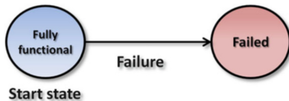
Fig. 2.3 A non-repairable system with two states
