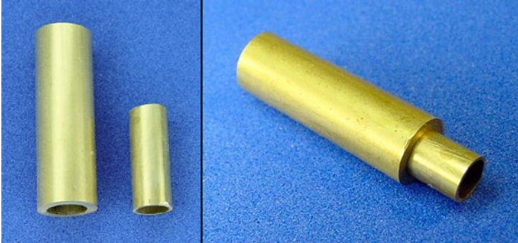
Figure 20-13. Left: Three 22 mm tubes inserted together (left side of left panel) placed beside a 13 mm tube (right side of left panel). Right: 13 mm tube partially inserted to test the fit
