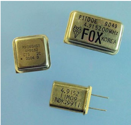
Figure 27-16. Half-can oscillator (middle left), full-can oscillator (top right), and crystal (bottom)
