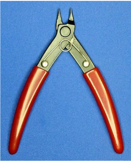
Figure 9-5. Flush wire cutter or nippy cutter
