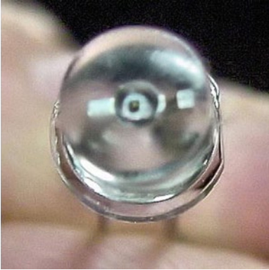
Figure 10-9. View of a reflector cup and die
