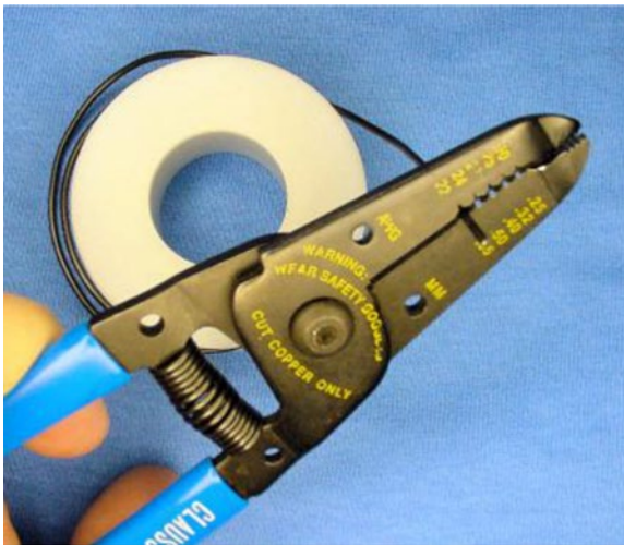
Figure 12-19. Numbered-notch wire strippers removing insulation from #22 AWG solid wire
