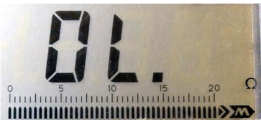
Figure 9-8. The resistor value is above the selected range on the multimeter
