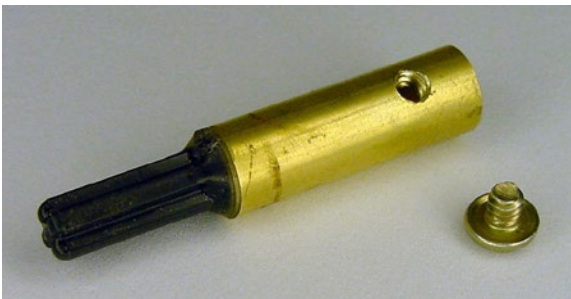
Figure 20-22. Finished coupler displaying beautiful screw threads. Alongside, a #4-40, \frac{1}{8} -inch long panhead machine screw
