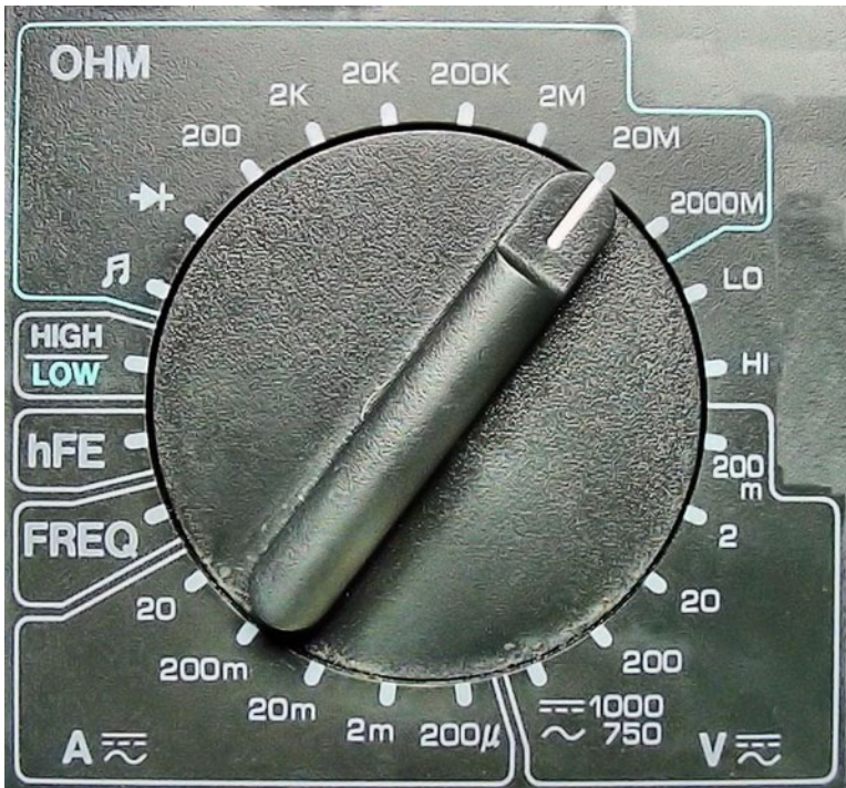
Figure 4-7. Dial with groups of manual range settings
