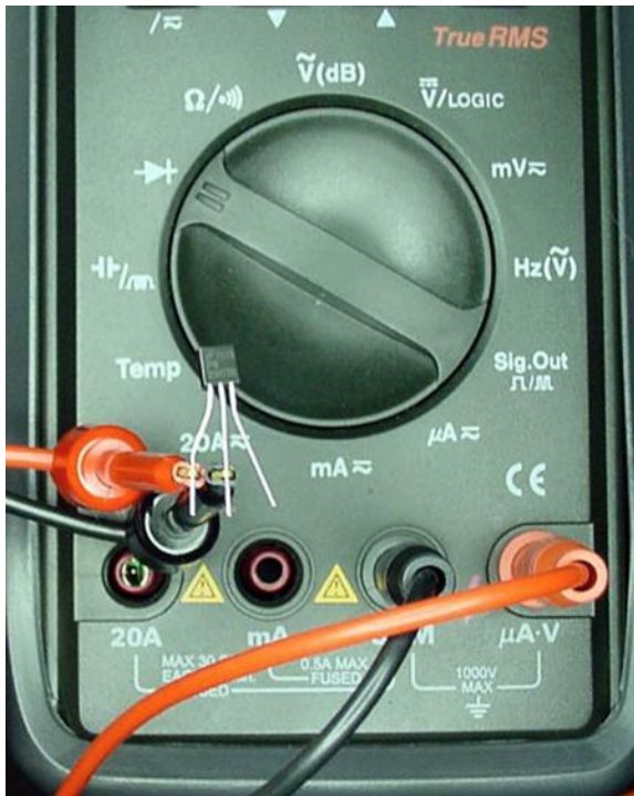
Figure 16-4. Setting up a multimeter for testing a transistor with the diode test function
