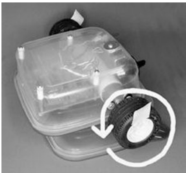
Figure 25-1. The robot’s left motor spins counter-clockwise. Notice the extra container underneath the robot keeping the wheels off the ground
