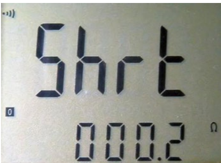
Figure 8-10. Multimeter displays short (connection) and almost zero resistance
