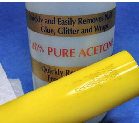
Figure 24-16. Removing sticker adhesive residue with acetone
