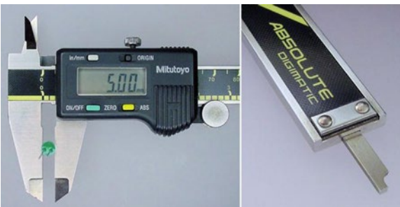
Figure 10-2. Measuring an LED diameter with calipers (left). The other end of the calipers protrudes for measuring the depth of a hole (right)
