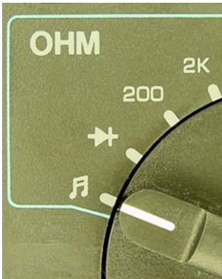
Figure 8-5. Multimeter dial set to continuity
