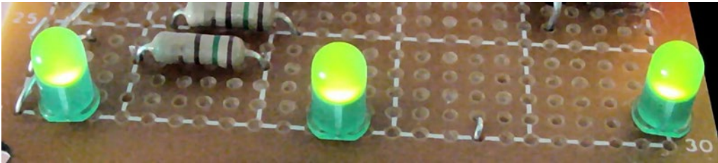
Figure 6-14. Brighter-left indicator LEDs as seen from left-side of robot
