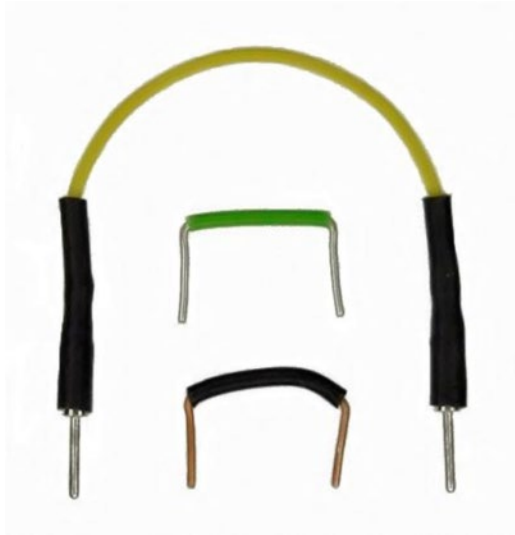
Figure 12-17. Jumper wire: Reinforced (top), ready-made (middle), handmade (bottom)
