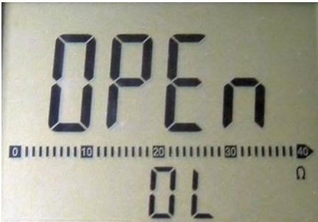
Figure 8-8. Multimeter displays open (no connection) and very high resistance
