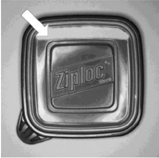
Figure 24-31. Window ground out of front of container lid
