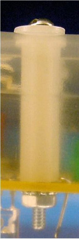
Figure 24-27. Mounting hardware installed. Top to bottom: screw head, washer, container, washer, spacer, circuit board, lock washer, nut, end of screw
