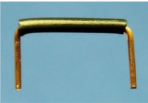
Figure 12-22. Completed homemade flat jumper wire
