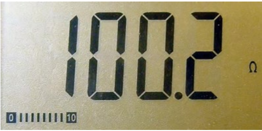
Figure 9-7. Meter displaying resistance of approximately 100 \Omega
