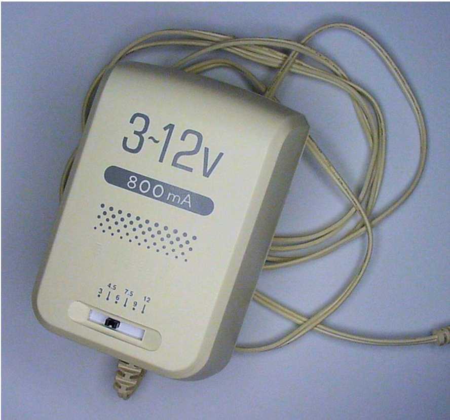
Figure 3-6. An AC-to-DC transformer with adjustable voltages from 3 volts to 12 volts
