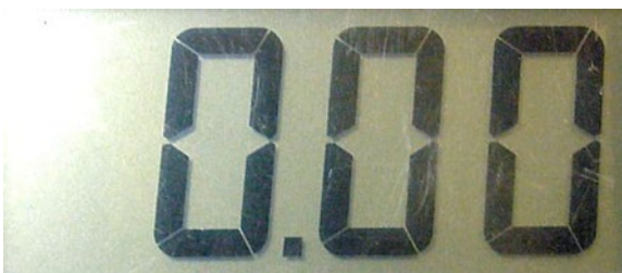
Figure 7-4. Meter displays no voltage
