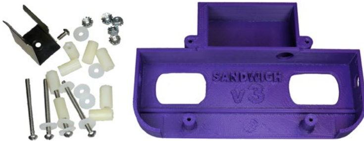
Figure B-2. All of these screws, nuts, washers, and standoffs are eliminated by incorporating those elements in the printed robot platform
