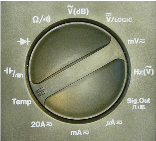
Figure 4-8. Dial simplified because of autoranging
