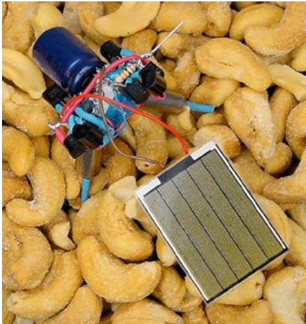
Figure 27-6. Appetizer, a BEAM robot, charging its rear capacitor from its front solar panel
