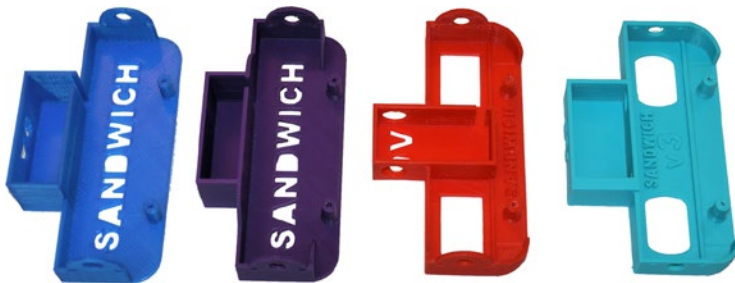
Figure B-20. A progression of design improvements on the 3D printed Sandwich robot platform
