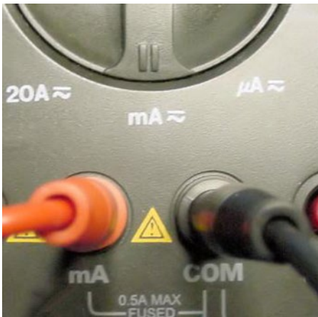
Figure 11-8. Multimeter setup for mA current flow
