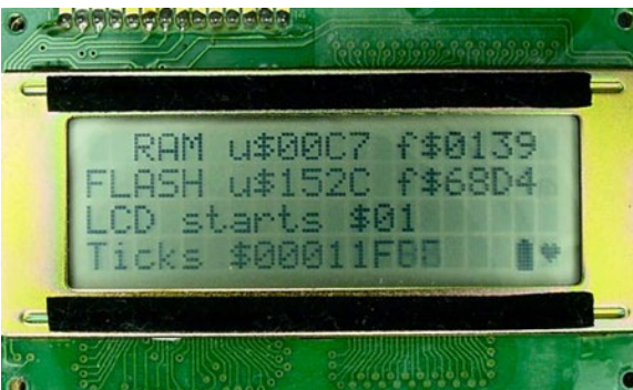
Figure 27-23. Standard 14-pin 20-character by 4-line LCD
