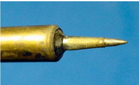
Figure 21-5. Fine tip of soldering iron
