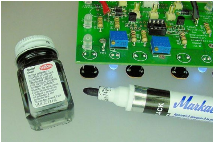
Figure 23-15. Black paint (left and bottom) and photocells raised 12 mm from circuit board surface (top right)
