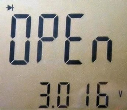
Figure 10-15. Open circuit indicating a test error or damaged LED
