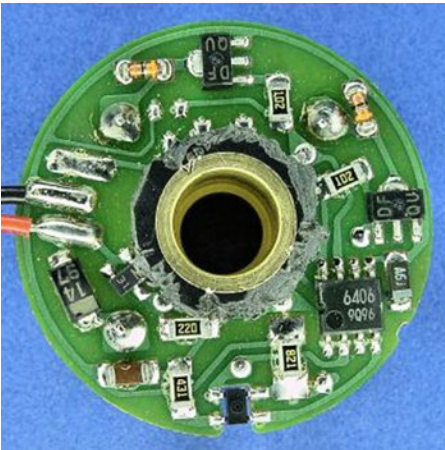
Figure 17-9. Circuit built into brushless motor
