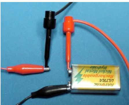
Figure 11-9. Power indicator circuit connection for current-flow measuring
