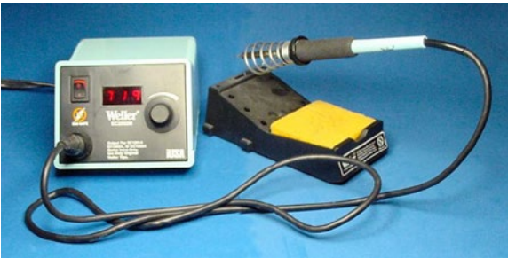
Figure 21-4. Temperature-adjustable soldering iron with sponge and stand
