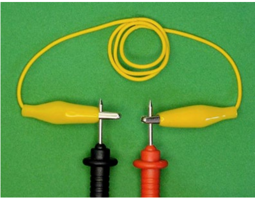
Figure 8-11. Making a connection with alligator jumper leads
