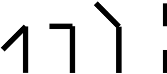
Figure 6-4. Unacceptably sharp turns: (left to right) 135^\circ , 90^\circ , and 45^\circ . (far right) broken line
