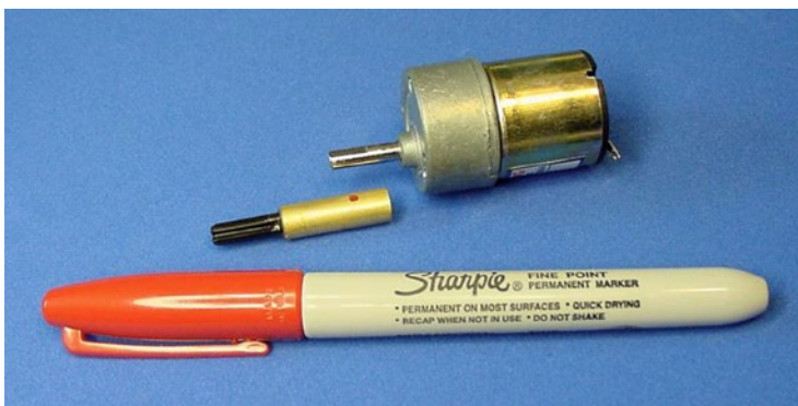
Figure 20-18. Marking desired location for the setscrew hole on a coupler using a fine-point permanent marker
