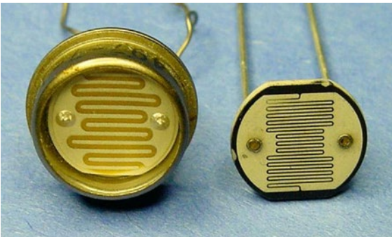
Figure 14-12. Encapsulated and exposed ceramic cadmium-sulfide photoresistors
