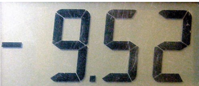
Figure 7-6. A negative number indicates a mixed-up connection
