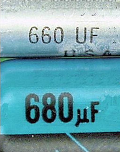
Figure 5-3. Some markings use the English letter “U” instead of the Greek letter “ \mu ”
