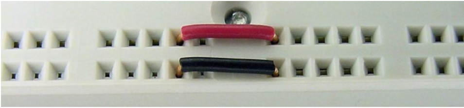
Figure 12-10. Extending buses by connecting with wire
