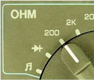
Figure 8-6. Multimeter dial set to lowest ohm range
