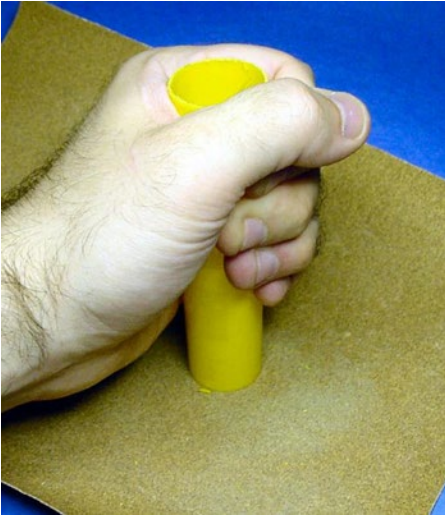
Figure 24-15. Removing burrs and shaping ends with a circular motion on sanding paper
