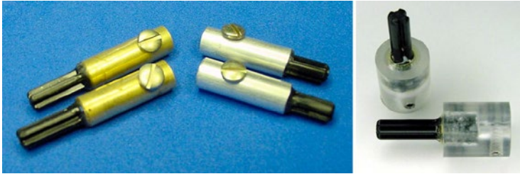
Figure 20-2. Two brass couplers (left) and two aluminum couplers (middle) made with tubing. Two plastic couplers (right) made on a lathe or milling machine out of solid rod
