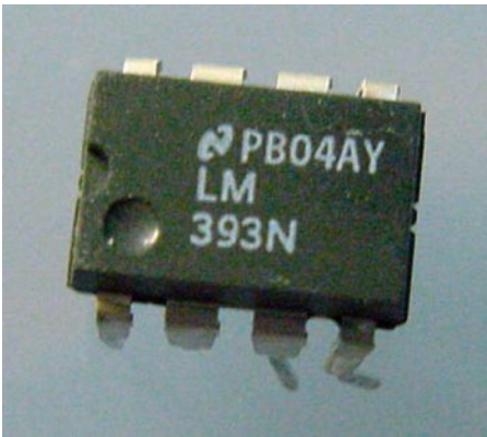
Figure A-3. A destroyed LM393N comparator
