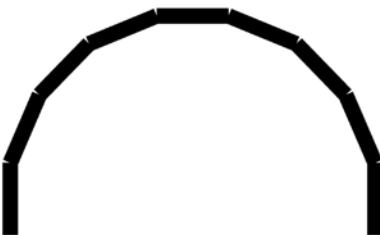
Figure 6-5. Acceptable 180^\circ turn made gradually from 22.5^\circ segments
