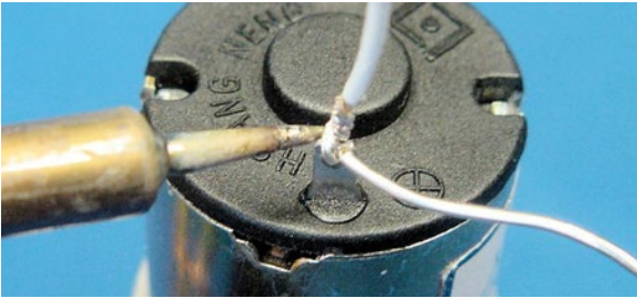
Figure 22-5. Soldering iron tip on one side of the wire, solder on the other side of the wire
