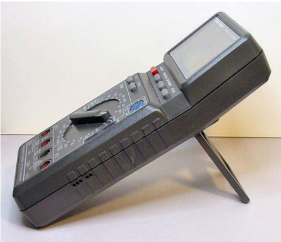
Figure 4-10. Multimeter held at readable angle by built-in stand
