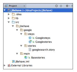
The steps class is clearly a Pojo. Pojo is short for a plain old Java object that does not extend any class and is literally called a Java class. It encloses the Java methods to be mapped with the aforementioned human-readable story file. Create a test step class using annotations provided by the JBehave API (Googlesteps.java):
