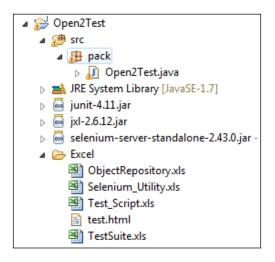
These components are available in the form of Excel sheets, where Utility Excel stores all the location paths of the object repository, test suite, test script, and report folder. The following table represents Selenium Utility Excel of the Open2Test framework:
