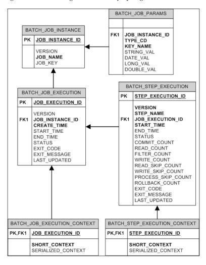
The following is the schema diagram defined by Spring Batch:
