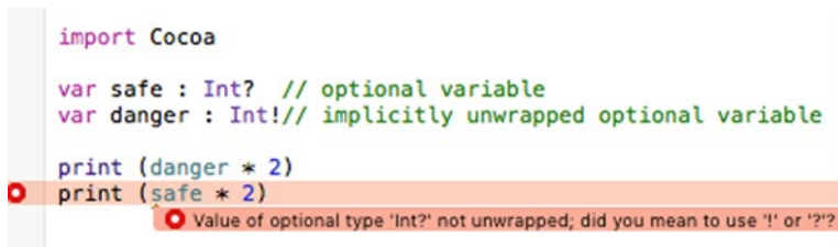
Figure 5-16. Xcode can identify possible problems with undefined optional variables but not undefined implicitly unwrapped optional variables
