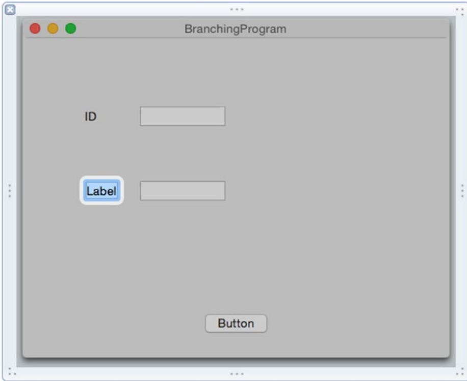
Figure 7-12. Double-clicking on a label lets you change the text without using the Attributes Inspector pane
