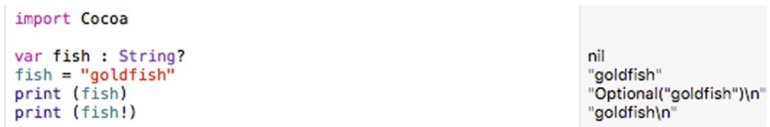
Figure 5-13. Seeing the difference between an optional and the unwrapped data inside an optional
