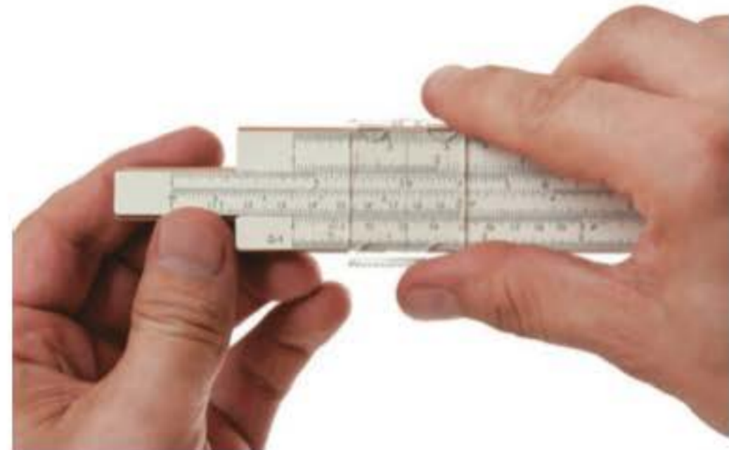
FIGURE 7-13 The slide rule was invented in the 17th century. The device uses logarithms to handle calculations. Engineers and scientists used slide rules into the 1950s and beyond.
