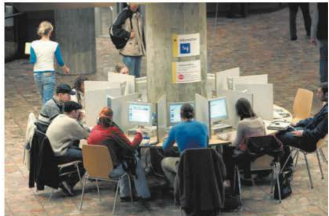
FIGURE 10-23 Although these workstations form a circle physically, the layout has no bearing on the network topology, which might be a bus, ring, star, or other logical design.
