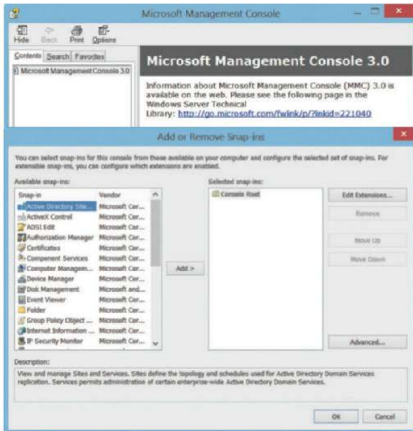
FIGURE 12-19 The Microsoft Management Console (MMC) includes built-in security tools, such as password and lock-out policies, audit policies, user rights, and security configurations, among others.
