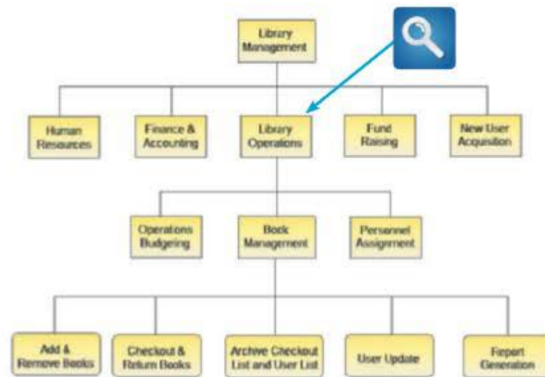
FIGURE 4-8 This Visible Analyst FDD shows a library system with five top-level functions. The Library Operations function includes two additional levels of processes and subprocesses.
