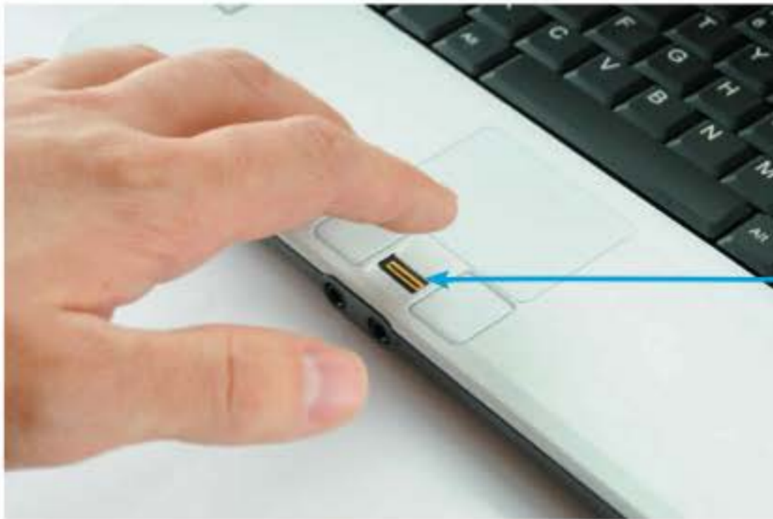
FIGURE 12-26 Some notebook computers feature a fingerprint reader, which is a small metallic sensor located near the keyboard or display.
