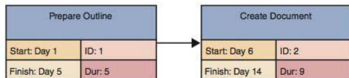
FIGURE 3-15 This example of a dependent task shows that the finish time of Task 1, Day 5, controls the start date of Task 2, which is Day 6.
