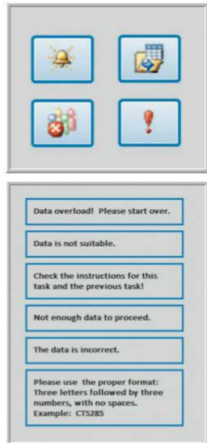
FIGURE 8-8 In the example at the top, the icons do not have a clear message. In the Help text examples at the bottom, only one message is understandable. The others would frustrate and annoy most users.
