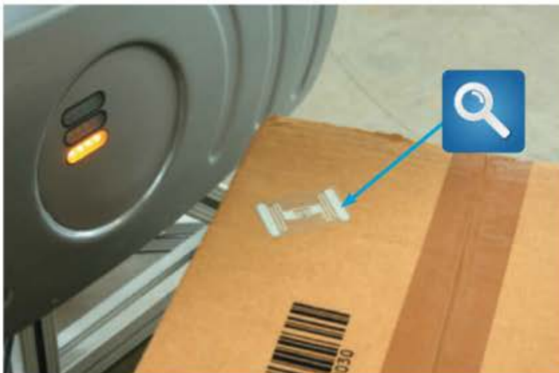
FIGURE 1-18 With an RFID tag, items can be tracked and monitored throughout the shipping process.
