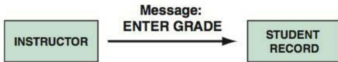
FIGURE 6-16 In a school information system, an INSTRUCTOR object sends an ENTER GRADE message to an instance of the STUDENT RECORD class.
