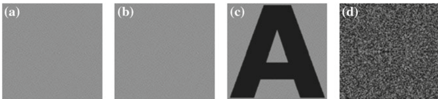
Fig. 2.9 Traditional visual cryptography decryption process. a Share one. b Share two. c Secret recovered by superimposing share two on share one. d Attempted secret recovery after flipping share two vertically and superimposing it on share one
