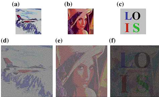
Fig. 5.2 Experimental results of the color (2, 2) -EVCS with pixel expansion of 4 in the visual cryptography model of Naor and Shamir (Size of the secret image is 200 \times 200 ) a Original two share image; b Original two share image; c Original secret image; d Encrypted shares; e Encrypted shares; f Resulting image by superimposing the shares ( d ) and ( e )
