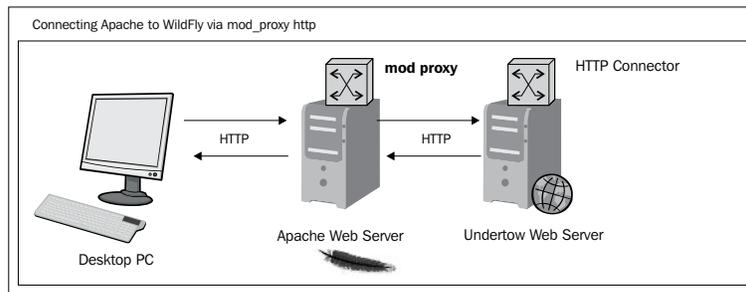
As shown in the preceding diagram, Apache's `mod_proxy` is TCP-based and uses HTTP, so you don't need to add anything else within your WildFly configuration. On top of this, there is also support for another module, `mod_proxy_ajp`. This module can be used in much the same way as `mod_proxy` except that it uses the AJP protocol to proxy Apache requests to WildFly. Before you can use it, you will need to enable it as follows:
