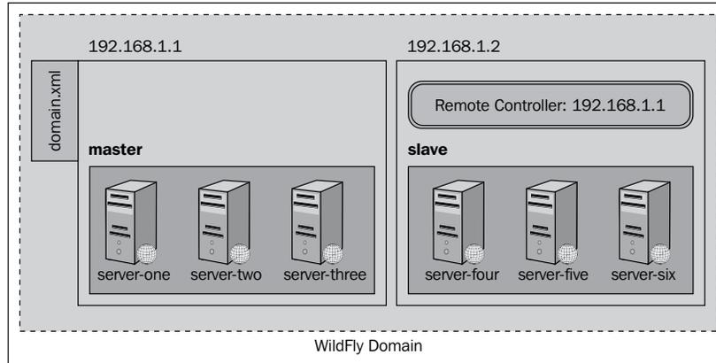
The first thing we need to do is bind the network interfaces to a valid `inet` address, both for the public and management interfaces. So, assuming that the first domain installation (master) will be bound to the `inet` address `192.168.1.1`, open the `host.xml` file and change it accordingly, as follows:
