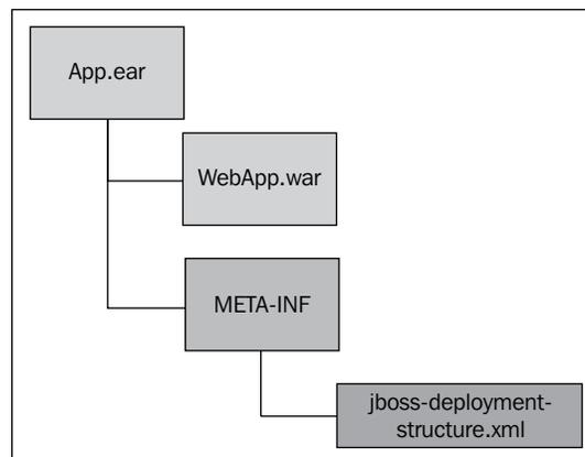
The following is the content of `jboss-deployment-structure.xml`:
