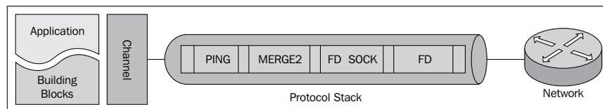
A JGroups process broadly consists of three parts, namely a **Channel**, the **Building Blocks**, and the **Protocol Stack**.
