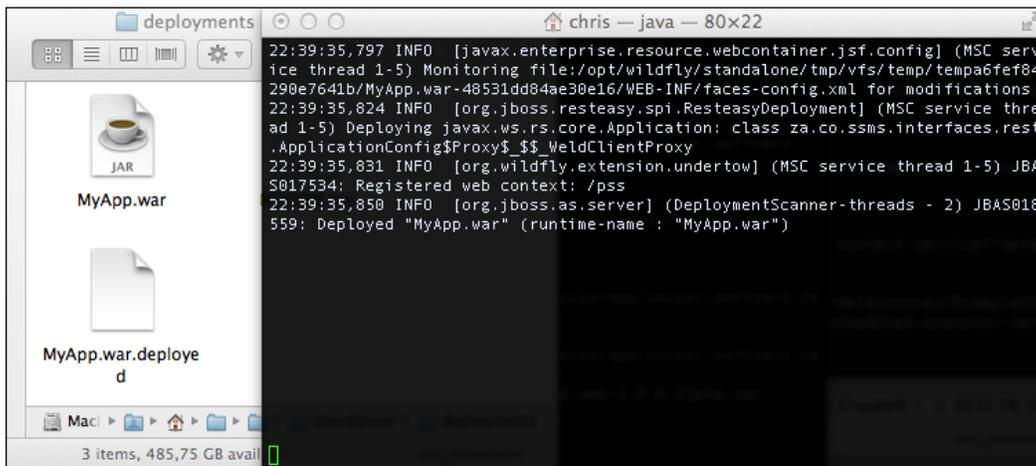
The service that scans for deployed resources is called the **deployment scanner**, and it is configured within the `standalone.xml` configuration file. You can find it by searching for the `deployment-scanner` domain. The following snippet shows the default deployment scanner configuration:
