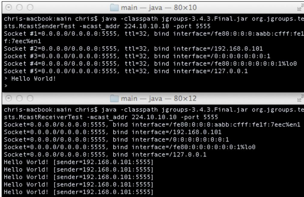
The screenshot shows two terminal windows. The top window, titled 'main — java — 80x10', shows the execution of `McastSenderTest`. It displays the command, socket binding details for five sockets, and the output 'Hello World!'. The bottom window, titled 'main — java — 80x12', shows the execution of `McastReceiverTest`. It displays the command, socket binding details for five sockets, and the output 'Hello World!' repeated five times, each with a sender address of 192.168.0.101:5555.
