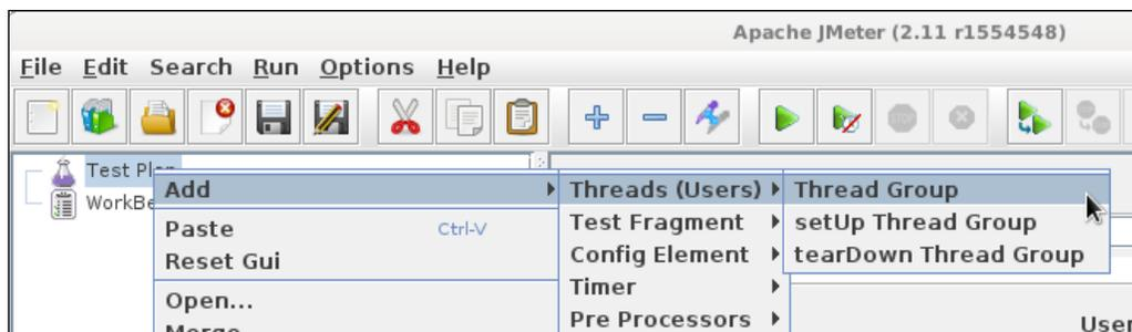
Set the number of threads (users) to 100. Now right-click on the newly created **Thread Group | Add | Sampler | HTTP Request**. In here, add the server IP and path, as shown to the right-hand side of the following screenshot. The port number can be left blank as it defaults to port number 80. Take a look at the following screenshot:
