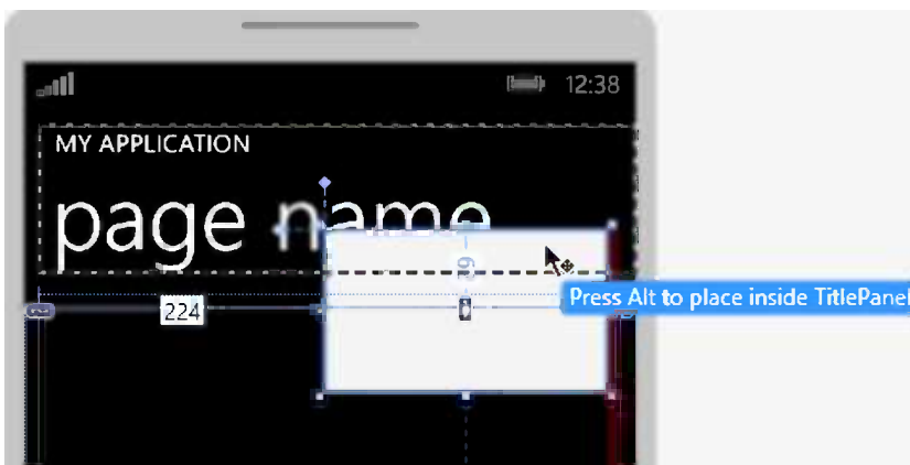
Figure 11-6. Dragging a control over the top of another container
