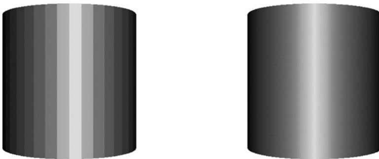
Figure 7-25. A cylinder with normals applied to each whole face (left) and to individual vertices (right)
