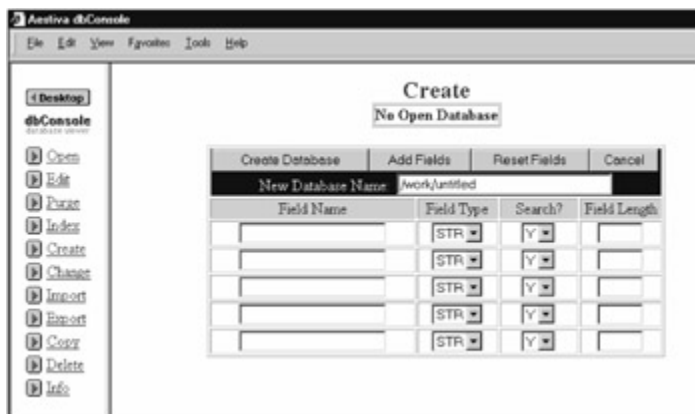
Figure 11.2: You Can Expand the Database Create Screen to Accommodate Additional Fields by Clicking the Add Fields Button.
