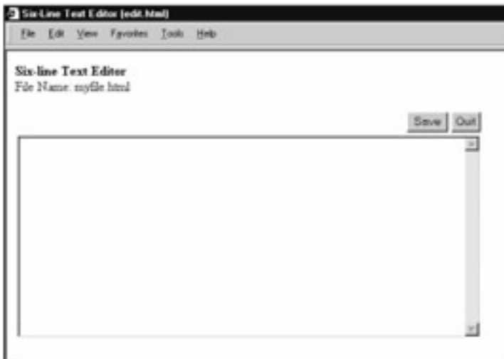
Figure 8.1: You Build the Six-Line Text Editor by using Six HTML/OS Instructions and Three HTML Form Components.
