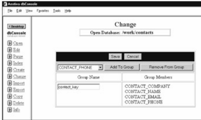
Figure 12.1: Use the Change Section in dbConsole to Add Group Fields to Databases.
