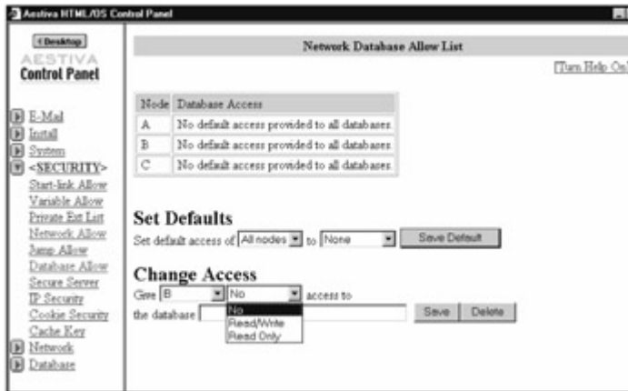
Figure 15.3: The Network Database Allow List Page of the HTML/OS Control Panel is Where You Place Limitations on Other Nodes Accessing Your Databases.
