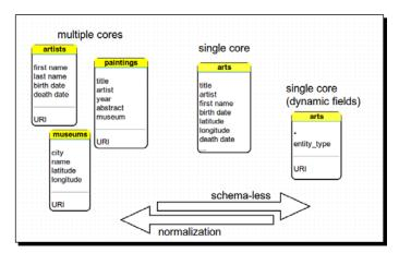
In the left part of this schema, we can find some suggested relationships between the different entities that could be used for joins if we were using a relational database. Note that Solr doesn't have a join functionality in the relational perspective as we have seen before, and it permits us to link together records representing different entity individuals by matching them on some criteria at runtime.
