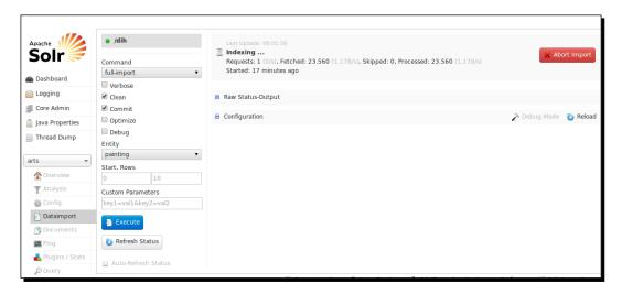
In this way, we can start a new import process by simply clicking the **Execute** button, as well as directly apply other parameters to enable cleaning of existing data, optimization, and so on. Here, the most important attribute is the choice of the import command by command=full-import. For example, another very useful choice would be delta import. You can still run almost the same command as usual by using cURL:
