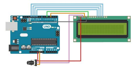
Follow these steps to connect an LCD to the Arduino:
