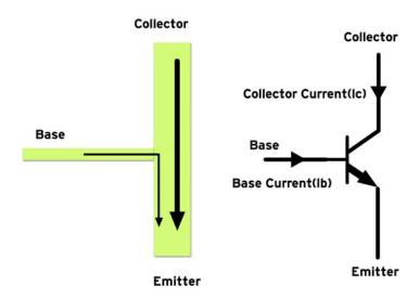
When we set the digital pin at HIGH on the Arduino, current passes from the pin to the base of the NPN transistor, thus allowing current to pass through the other two terminals. When we set the pin at LOW, no current goes to the base and so, no current will pass through the other two terminals. Another analogy would be a digital switch that allows current to pass from the collector to the emitter only when we 'push' the base with current.
