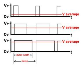
We can see in the first part of the graphic that we are mostly keeping the pin LOW, to 0 V, and thus the average voltage output is quite low. In the middle of the graphic, we are roughly keeping the pin HIGH and LOW for an equal amount of time, and the resulting voltage is half. In the last part, we see that the time the pin is HIGH is called Pulse Width. The total time between the beginning of each pulse is called the period of the PWM signal.
