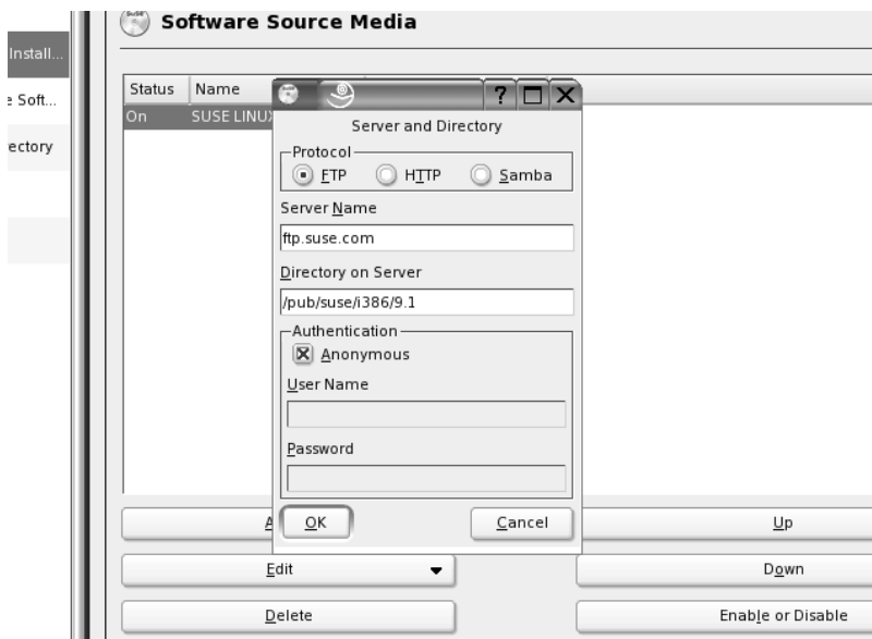
Figure 29-3. You may want to add the main SUSE FTP site as an installation source if you won't always have the DVD on-hand.
