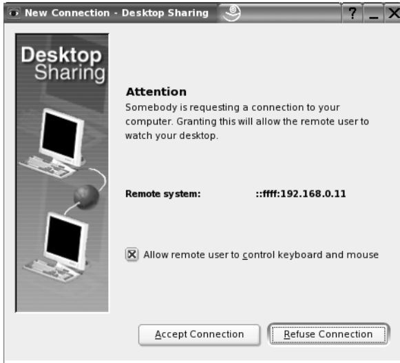
Figure 34-4. Before the remote user can connect, you'll need to agree to that user having access.
