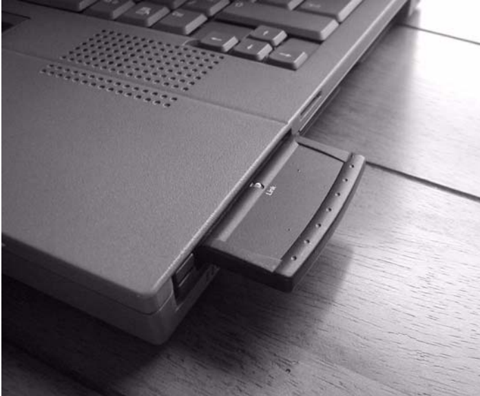
Figure 8-3. Most wireless cards rely on an aerial of some kind.
