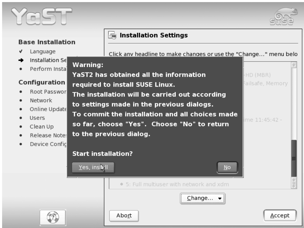
Figure 5-8. When you're happy with the installation choices, click the Yes, Install button to start copying files.
