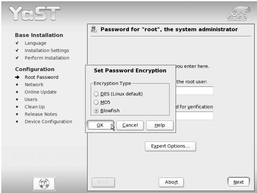
Figure 5-11. SUSE Linux defaults to eight-character passwords, but you can change this by selecting a different encryption method.
