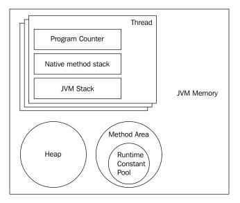
The JVM contains the native code and the Java bytecode to be provided to the Java API implementation and the JVM implementation. The native code call stack is maintained separately for each thread stack. The JVM stack contains the Java method calls. Please note that the JVM spec for Java SE 7 does not imply a native method stack, but it does for Java SE 5 and 6.
