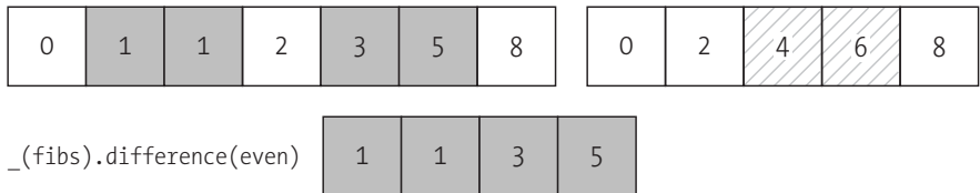
FIGURE 8-9: The difference() function returns elements that are present only in the first of multiple arrays.
