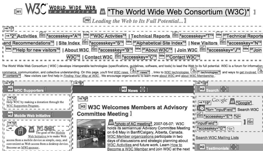
Figure 4.3: WebAIM's WAVE Web Accessibility Tool Overlays a Page with Testing Result Icons
