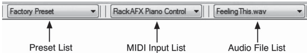
Figure 2.4: The drop-down boxes on the right let you store and recall Presets, choose a MIDI input Controller, and keep track of the audio files you have been using.
