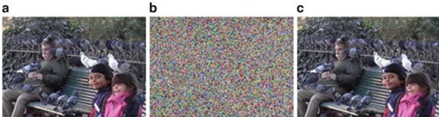
Fig. 18.6 (a) Original jpg image message to be sent for computer A, (b) hyperchaotic encrypted image through insecure channel, and (c) recovered jpg image for computer B
