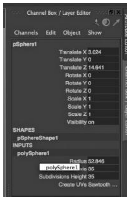
FIGURE 2.13 The input node allows changes to the shape to be made, as long as the history is intact.
