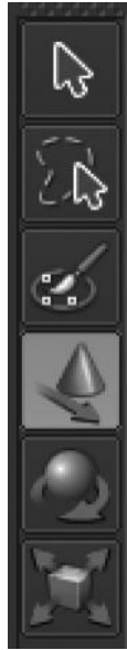
FIGURE 1.17 The Tool Box where you can select, translate, rotate, or scale objects.
