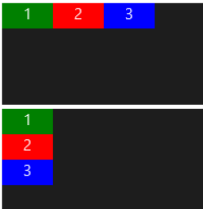
FIGURE 3-9 The two divs with a FlexBox layout; the top one shows a row direction, and the bottom one shows a column direction
