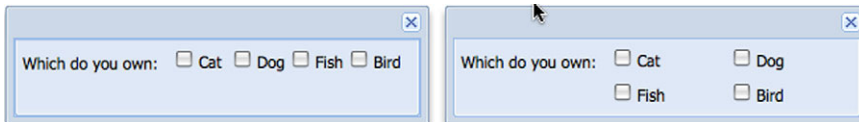
Figure 6.14 Two implementations of the checkbox group: single horizontal line (left) and a two-column layout (right)
