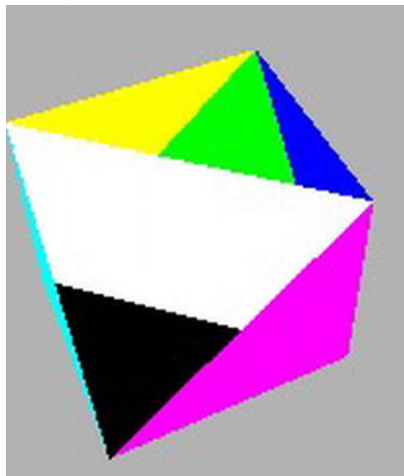
Figure 7-10. Not enabling the depth test can produce strange results
