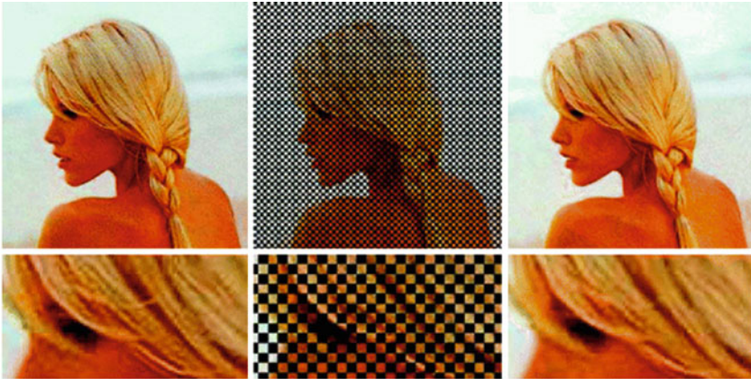
Original color image ( left ), image with 50% pixel removed ( middle ), reconstructed using PDE (50.75) ( right )
