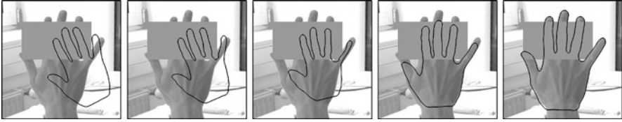
Fig. 6 Gradient descent evolution of a parametric curve from initial to final with similarity-invariant shape prior. The statistical shape prior permits a reconstruction of the hand silhouette in places where it is occluded
