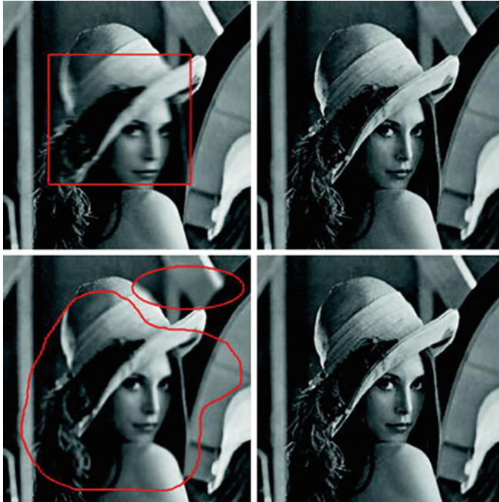
Fig. 19 Non-blind space-variant restoration. Left column: spatially variant motion blurred images. Right column: the corresponding recovered images using the suggested method
