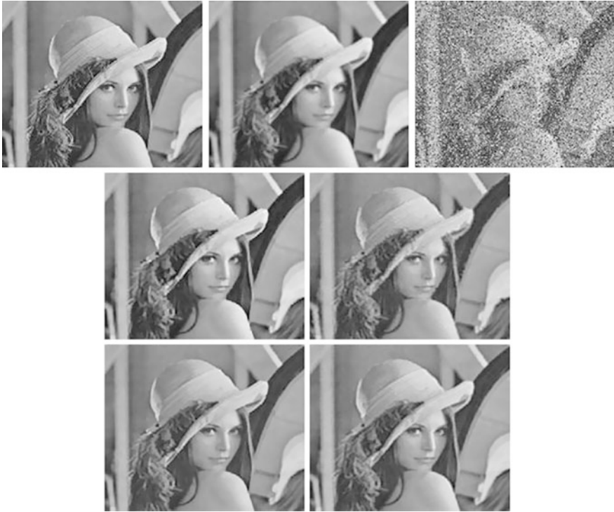
Fig. 25 Recovery of noisy-blurry image with Gaussian kernel with \sigma = 1 and salt-and-pepper noise with d = 0.3 . Top row : original image, blurry image, noisy-blurry image. Middle row : recovered images using MSTV (SNR = 27.8336), MSH 1 (SNR = 23.2052). Bottom row : recovered images using NL/MSTV (SNR = 29.3503), NL/MSH 1 (SNR = 27.1477). Parameters : \beta = 0.25 (MSTV), 0.1 (NL/MSTV), \alpha = 0.01 , \varepsilon = 0.002 . Parameters : \beta = 2 (MSH 1 ), 0.55 (NL/MSH 1 ), \alpha = 0.001 , \varepsilon = 0.0001
