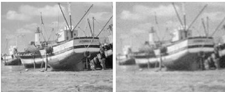
Fig. 23 Original and noisy-blurry images (noisy-blurry image using the pillbox kernel of radius 2 and Gaussian noise with \sigma_n = 5 )
