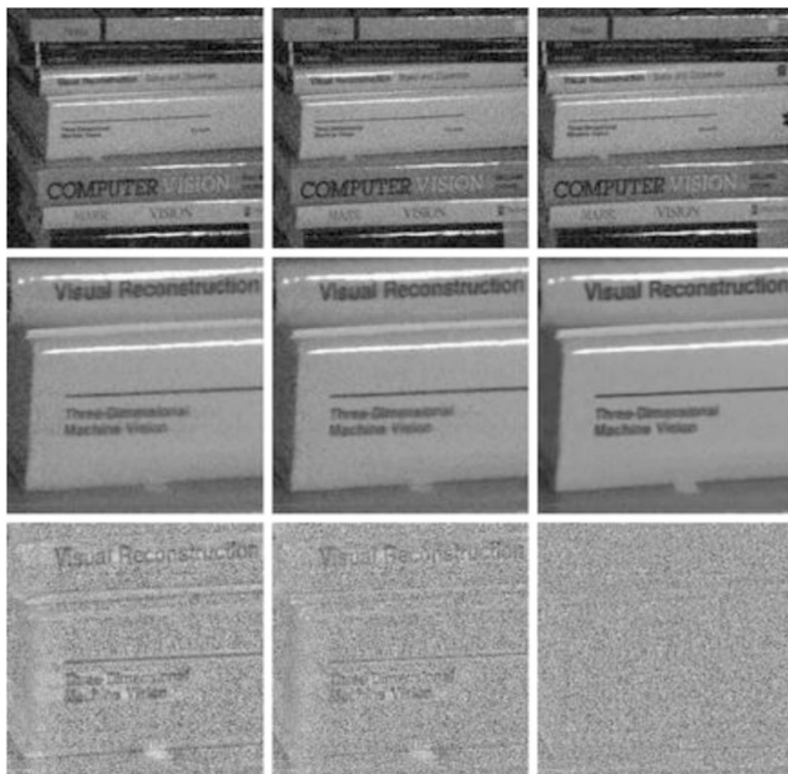
Fig. 13 Comparison of static filters, motion compensated filters, and NL-means applied to an image sequence. Top : three frames of the sequence are displayed. Middle and left to right : neighborhood filter, motion compensated neighborhood filter, and the NL-means. (AWA). Bottom : the noise removed by each method (difference between the noisy and filtered frame). Motion compensation improves the static algorithms by better preserving the details and creating less blur. We can read the titles of the books in the noise removed by AWA. Therefore, that much information has been removed from the original. Finally, the NL-means algorithm ( bottom row ) has almost no noticeable structure in its removed noise. As a consequence, the filtered sequence has kept more details and is less blurred
