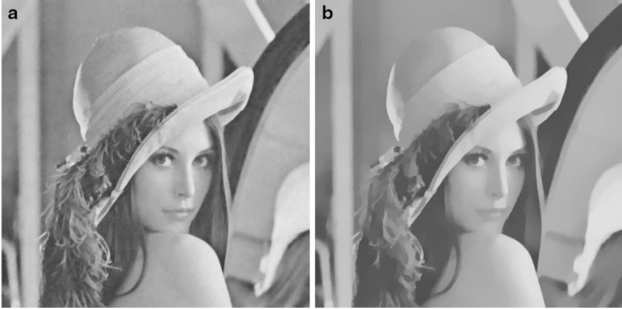
Fig. 7 (a) Left : the result obtained by computing E(u|f) and \beta\sigma^2 = \lambda = 20 , \sigma = 10 (image courtesy of Cécile Louchet). (b) Right : the result obtained using Chambolle's algorithm with \lambda = 20
