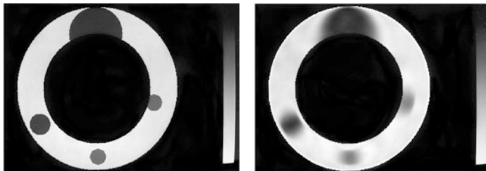
Fig. 2 Exterior reconstruction. Phantom ( left ) and reconstruction ( right ) from simulated data [77, ©IOP Publishing. Reproduced by permission of IOP Publishing. All rights reserved]. The outer diameter of the annulus is 1.5 times the inner diameter
