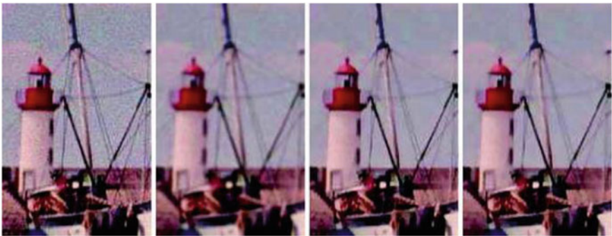
Fig. 2 From left to right: noise image, Gaussian convolution, neighborhood filter, and bilateral filter. The neighborhood and bilateral filters avoid the excessive blurring caused by a Gaussian convolution and preserve all contrasted edges in the image
