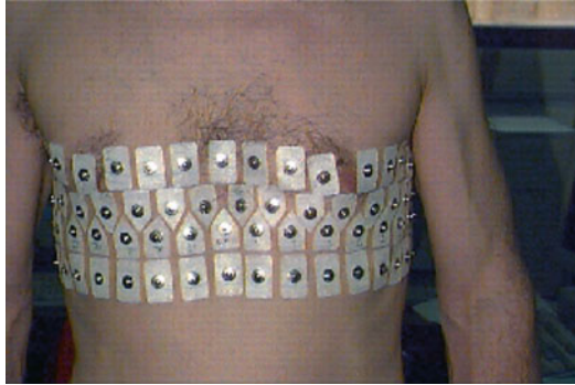
Fig. 2 A system of electrodes used for chest EIT at Oxford Brookes University. The positions of the electrodes were measured manually with a tape measure and the cross-sectional shape was also determined by manual measurements. These electrodes have a disk of jell containing silver chloride solution that makes contact with the skin. Each electrode was attached to the EIT system by a screened lead, not shown in this picture for clarity
