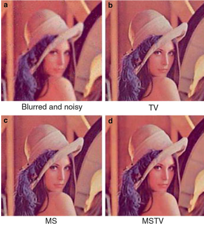
Fig. 18 Recovery of the Lena image blurred by 7 \times 7 out-of-focus kernel contaminated by mixture of Gaussian and salt-and-pepper noise
