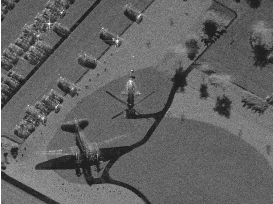
Fig. 17 A 4-in. resolution image from Sandia National Laboratories. Note the shadows of the historical airplane, helicopter, and trees (Courtesy of Sandia National Laboratories)
