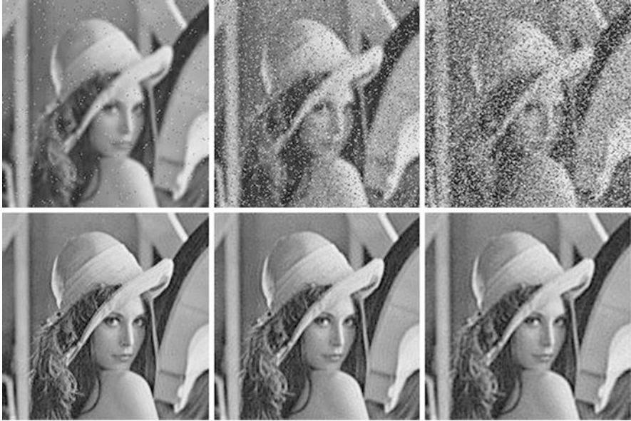
Fig. 15 Top row: the Lena image blurred with a pillbox kernel of radius 3 and contaminated by salt-and-pepper noise. The noise density is ( left to right ) 0.01, 0.1, and 0.3. Bottom row: the corresponding recovered images
