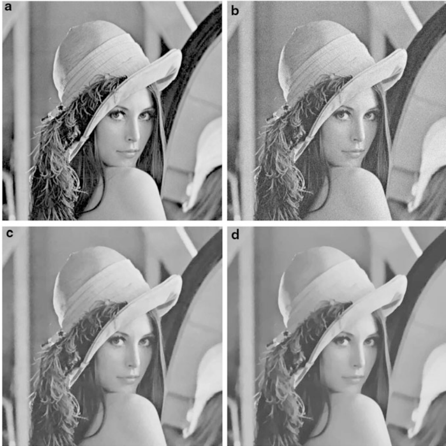
Fig. 2 Denoising results obtained with Chambolle’s algorithm. (a) Top left : the original image. (b) Top right : the image with a Gaussian noise of standard deviation \sigma = 10 . (c) Bottom left : the result obtained with \lambda = 5 . (d) Bottom right : the result obtained with \lambda = 10
