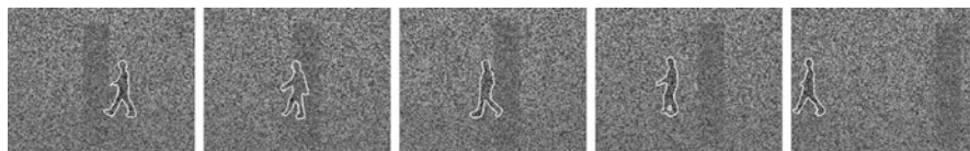
Fig. 17 Tracking in the presence of occlusion. The dynamical shape prior allows to reliably segment the walking person despite noise and occlusion
