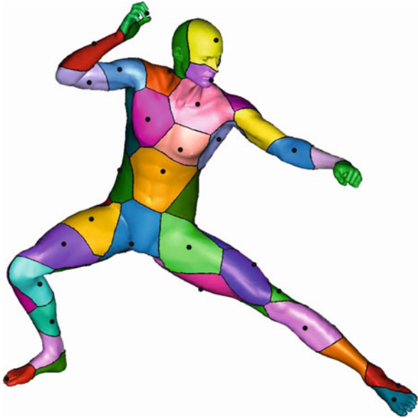
Fig. 2 Voronoi decomposition of a surface with a non-Euclidean metric
