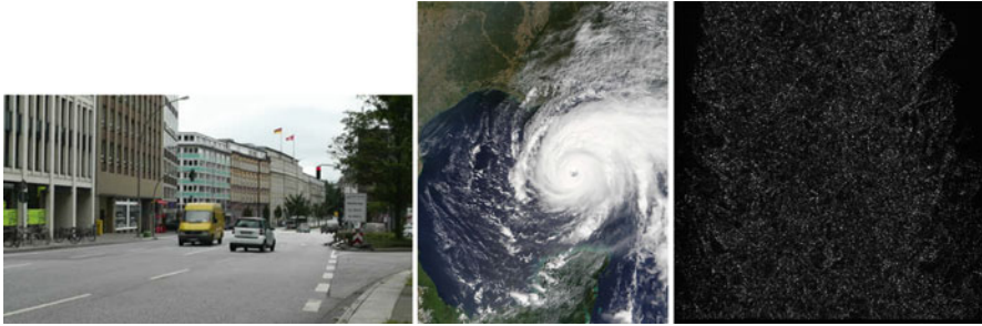
Fig. 1 Some application areas of image processing that essentially rely on image motion analysis. Left : scene analysis (depth, independently moving objects) with a camera mounted in a car. Center : flow analysis in remote sensing. Right : measuring turbulent flows by particle image velocimetry
