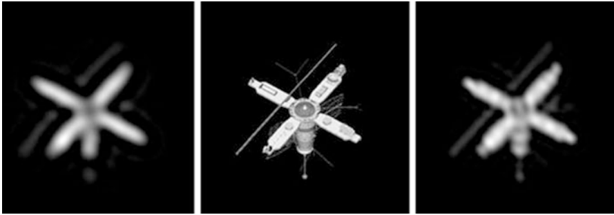
Fig. 11 On the left is the initial reconstructed image using \mathbf{x}_0^{(n\ell)} and on the right is the final reconstructed image. The true image is displayed in the middle for comparison purposes
