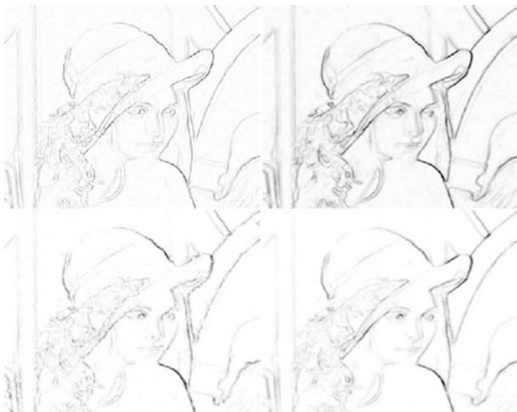
Fig. 26 Edge map \nu using the MS regularizers in the recovery of the Lena image blurred with Gaussian blur kernel with \sigma_b = 1 and contaminated by salt-and-pepper noise with density d = 0.3 . Top: (left) MSTV, (right) NL/MSTV. Bottom: (left) MSH 1 , (right) NL/MSH 1
