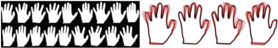
Fig. 15 First four modes of variation with ratios \frac{\lambda_i}{\lambda_1} of 1, 0.88, 0.42, and 0.25 for the 18 hand silhouettes from Fig. 10
