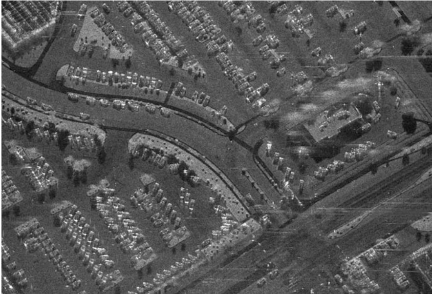
Fig. 15 A Ku-band image showing streaking due to objects moving in the scene (Courtesy Sandia National Laboratories and SPIE)
