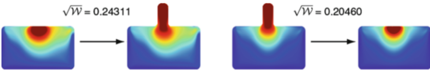
Fig. 7 The state-based elastic dissimilarity measure d_{\text{elast}} is not symmetric (as opposed to the path-based, viscous distance d_{\text{viscous}} ): In this example, it costs much more energy to drag out the protrusion than to push it in. The color coding represents the local deformation energy density in the reference and the deformed configuration
