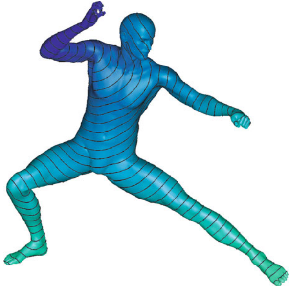
Fig. 4 Distance map measured on a curved surface. Equidistant contours from the source located at the right hand are shown (Reproduced from [25])
