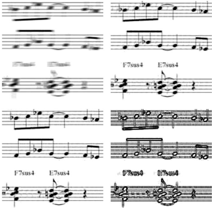
Fig. 10 The case of a known (nine-pixel horizontal motion) blur kernel. Top left : corrupted image. Top-right : restoration using the TV method [70, 80]. Bottom left : restoration using the MS method. Bottom right : edge map produced by the MS method
