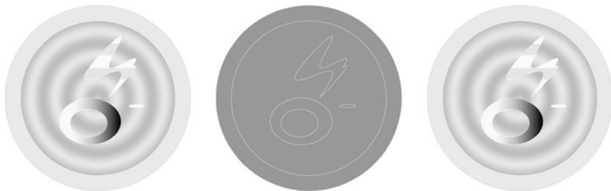
Fig. 8 Reconstruction test. From left to right , the conductivity distribution, the initial guess, and the reconstructed conductivity after three iterations
