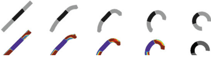
Fig. 21 Discrete geodesic between the straight and the folded bar from Fig. 19, where the black region of the initial shape is constrained to be matched to the black region of the final shape. The bottom row shows a color coding of the corresponding viscous dissipation. Due to the strong change in relative position of the black region , the intermediate shapes exhibit a strong asymmetry and high dissipation near the bar ends
