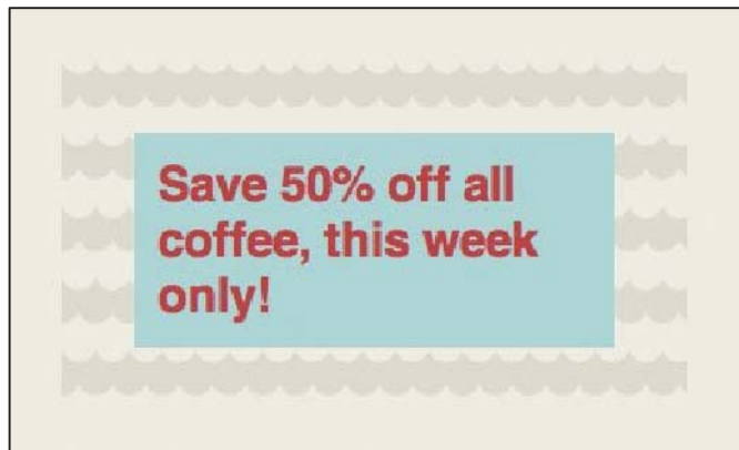
Figure 3.8 How the example might look in browsers that don't support RGBA or border-radius .
