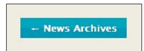
Figure 2.34 The button as rendered in IE7 (or any other browser that doesn't support border-radius ).
