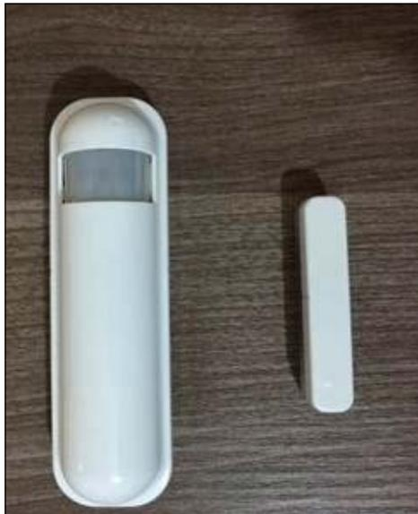
As shown in the preceding image, on the Philio multi-sensor device, you will also see a motion sensor at the head of the bigger part of the device. Motion sensors can also be used separately and you can place them in various places to detect motion.
