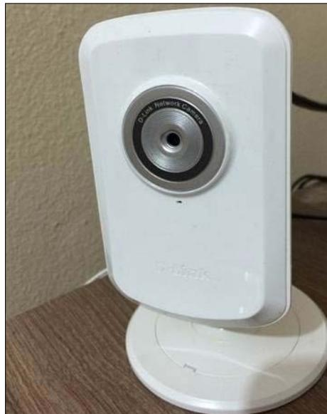
Some network cameras have a few built-in functions to be used for the security of your home. These built-in functions could be motion detection and sound detection. In accordance with the defined function, it can send a frame to the defined email client.
