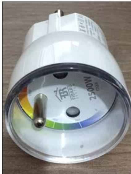
We will try to switch it on and off by sending basic commands through a Z-Wave controller. We will use the **Aeon Labs Z-Stick S2** USB adapter for our controller. As Intel Galileo has a USB host port, we will connect the Z-Wave controller from Intel Galileo's USB host. The Z-Wave USB adapter uses serial communication when it's on a host device, and so we will implement a couple of C functions to create communication with the device. You can see the USB adapter in the following image:
