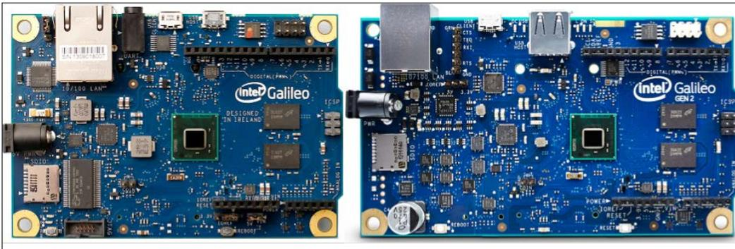
The first board (on the left-hand side) is the Intel Galileo Gen 1 version and the second one (on the right-hand side) is Intel Galileo Gen 2.
