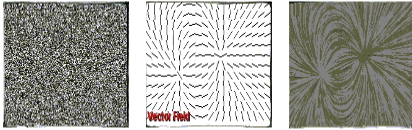
Figure 5.14. The texture field on the left is combined with the vector field in the middle to create the line integral convolution on the right. (Images generated with LicFactory [423].)
