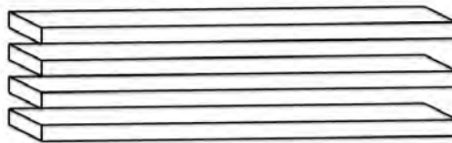
Figure 3.2. Four \neq three. As in Figure 3.1, this object would have a problem being built (there are four boards on the left and three on the right).
