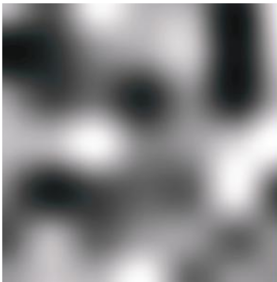
Figure 2.2. Nonlinear interpolation of a 5 \times 5 grid of random values provides smooth transitions between adjacent points.
