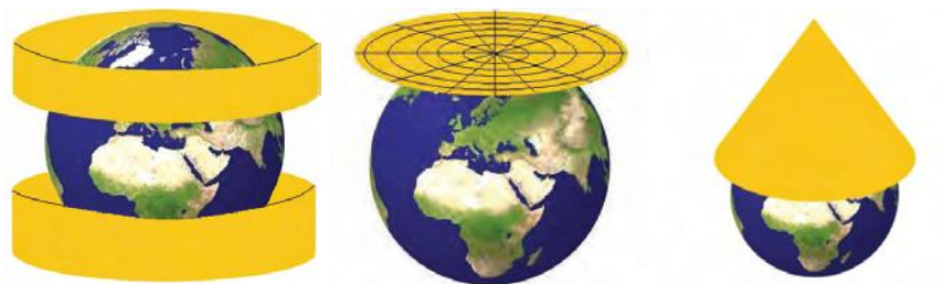
Figure 6.1. Cylinder, plane, and cone projections.
