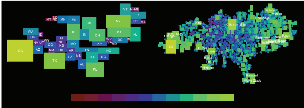
Figure 6.22. A rectangular U.S. population cartogram on the state and county level. The area of the rectangles corresponds to the population and the color redundantly encodes the population numbers. (Image from [157], © 2004 IEEE.)
