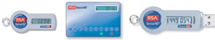
FIGURE 20.13 RSA SecurID tokens that provide one-time passwords. (Courtesy of RSA Security.) The left one is designed for a user to type the passcode displayed on the token; the center one allows a user to type in a PIN to the token and then a passcode will be generated for a user to type into a computer or smart phone. The right one has a USB interface and can send a password directly to a computer.
