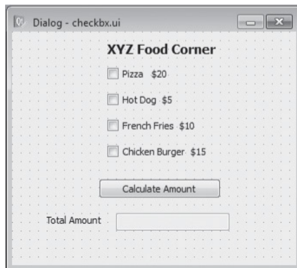
Figure 8.3. Form with four checkboxes, a push button, and a LineEdit widget in disabled mode.
