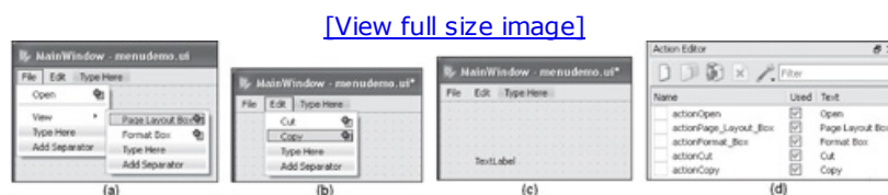
Figure 10.3. (a) Adding submenu entries to the View menu entry. (b) Cut and Copy menu entries added to the Edit menu. (c) A Label widget added to indicate which menu entry is selected. (d) All menu entries represented as actions in Action Editor.
