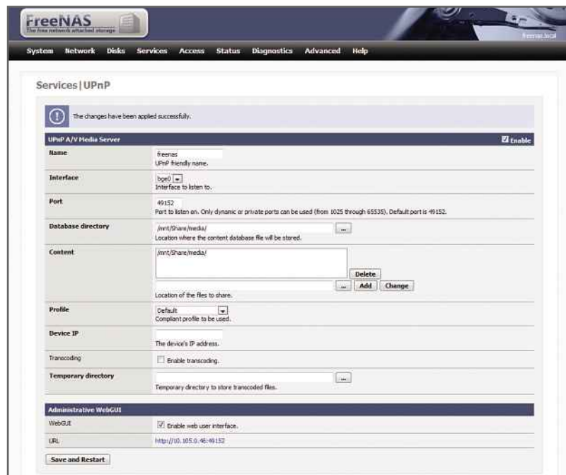
Your FreeNAS computer can share media files using its built-in UPnP server
