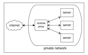
This is the type of proxy we might use to balance requests from clients across many Node servers. Client *X* does not communicate with any given server directly. A broker *Y* is the point of first contact, able to direct *X* to a server that is under less load, or that is located closer to *X*, or is in some other way the best server for *X* to access at this time.
