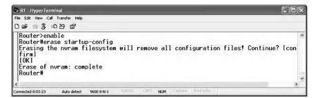
Use the "reload" command to reload the system and then disable the DNS lookup and Synchronize logging messages as shown in the following commands:
