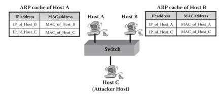
After the attack, the following figure shows the invalid entries in the ARP caches of Hosts A and B.
