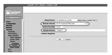
Next, create an attack group, as shown in the screenshot below. An attack group includes all the attack signatures that the Deep Inspection process will use in a given filtering rule. Therefore, an attack group may include more than one attack signature. In the case of the above security policy (SP#1), only one attack signature is used.
