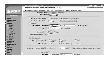
Click on the "Edit" link of bgroup0 interface and fill in the entries. The zone name will be "Trust" for the Dubai site and the interface mode is "NAT." Enable the services as was done for the Al-Ain site. Then click "Apply" and "OK."
