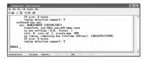
The output of the above command indicates that the number of encapsulated, encrypted, and digested packets is 11. The number of decapsulated, decrypted, and verified packets is 10. The number of compressed and decompressed packets is 0. The IPsec mode is the tunnel mode. There are two SAs, one inbound and one outbound. Every SA has its own SPI. A similar output will appear for the Dubai site, as in the following:
