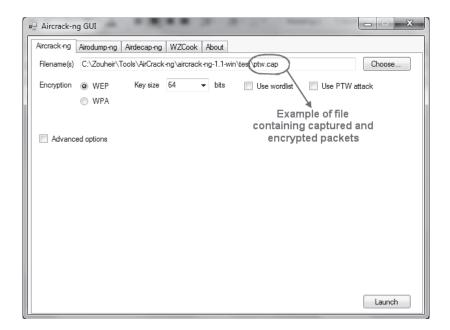
The following screenshot shows the result of cracking a WEP key using the Aircrack-ng tool. The WEP key found is "1F:1F:1F:1F:1F:1F."
