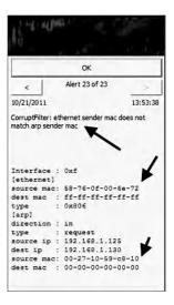
The XArp 2 CorruptFilter alert message indicates that the ARP packet includes incorrect values. That is, the Ethernet source MAC address does not match the ARP source MAC address. XArp 2 checks these values for correctness.
