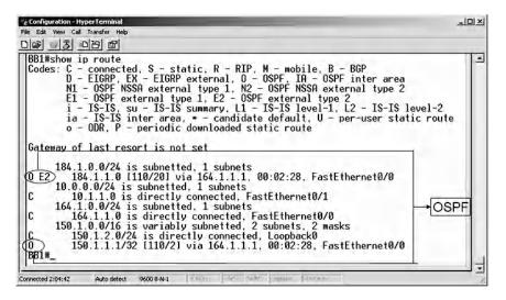
Test the connectivity of the network by pinging the inside PC from router BB1, which is successful because BB1 learns about the inside network from OSPF routing table entries.
