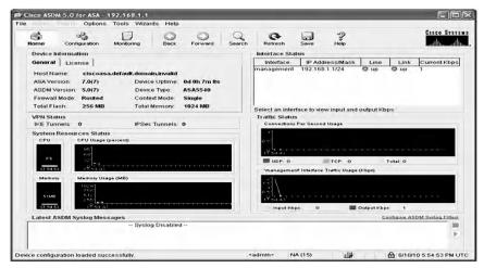
Click on the "Configuration" tab to get a display of all the interfaces of the firewall as shown in next screen.
