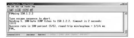
Next, ping the outside PC from router FW. This should be successful because the OSPF protocol is enabled.
