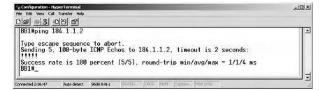
Then ping the loopback interface, which should be successful.
