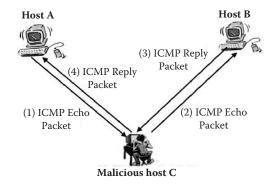
At Host C, *CommView sniffer* is used to capture the four exchanged packets. The analysis of the source and destination MAC addresses of the four captured packets clearly indicates that the exchanged ping traffic between Host A and Host B has been forwarded to Host C.
