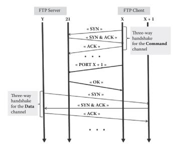
In addition, because FTP uses TCP-based channels, for each channel, four filtering rules are required to allow the corresponding traffic to pass through the firewall. For example, if the FTP client is an internal host and the FTP server is an external host, then the two subsequent tables list all the necessary filtering rules for the Command and Data channels, respectively.
