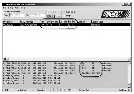
The major limitation of this detection technique is that if a sniffing host stops responding to ARP request messages while sniffing the network traffic, using, for example, a local firewall, then the technique becomes useless because it relies on the ARP response messages generated by the sniffing host.
