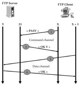
7.7.3.1 Passive FTP Traffic Filtering
