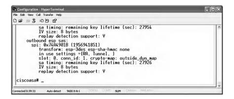
It is noticed that the current number of encapsulated, encrypted, and digested packets is 0; the number of de-capsulated, decrypted, and verified packets is 255; the number of compressed and decompressed packets is 0; the IPsec mode is the tunnel mode; and there are two SAs, one inbound and one outbound and each SA has its own SPI. To view more details of the VPN tunnel, type the following command:
