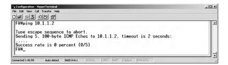
Finally, ping from the inside PC to the outside PC. This should not be successful because of the absence of a dynamic routing protocol, as in the following command:
