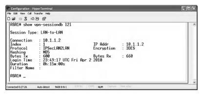
Several parameters of the session that occurred between the peers are displayed, such as Session Type: LAN-to-LAN. The connection is established with the other peer 10.1.1.2. The encryption and hashing algorithms are displayed, and the login time and the duration of the session are also displayed. Similar output can be obtained for the Dubai site as in the following:
