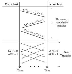
Therefore, if we consider only the SYN and ACK flags, there are only four types of TCP packets exchanged in a TCP connection:
