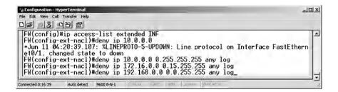
2. *Security policy: Implement RFC 2827 and log using ingress traffic filtering.* To prevent a DoS attack that employs spoofed IP source addresses, a security measure must be implemented to block packets that claim to have IP source addresses similar to the internal network.
