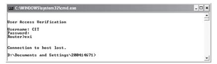
Sniff the Telnet packets on port 23. As demonstrated in the following series of screenshots, the Telnet traffic is not encrypted. By analyzing the traffic, it is easy to capture the Telnet username and password, which appear character by character. The TCP packet number 5, as shown in the next screenshot, contains the user access verification message prompt.
