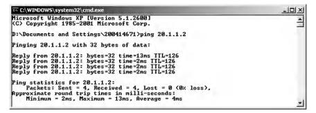
Ping from Dubai to Al-Ain, which should be successful. This confirms that the VPN tunnel is established in both directions.
