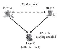
Then, using the ARP cache poisoning technique, the malicious user corrupts the ARP caches of the two target hosts, in order to force the two hosts to forward all their packets to the malicious host. This is extremely potent when we consider that not only can hosts be poisoned, but routers/gateways as well. All Internet traffic for a host could be intercepted by performing a MiM attack on the host and the LAN's router.
