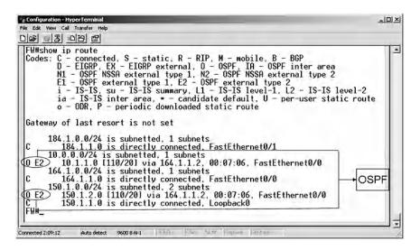
Configure dynamic routing on router BB1 by repeating the previous step for router FW but with corresponding network IP addresses, as in the following command:
