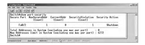
The following screenshot clearly shows that Host A has lost its connection to the switch (the interface 0/2 has been shut down), and a warning message has appeared on Host A's desktop.
