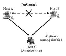
The MiM attack as shown above (i.e., second previous figure), where Host C is the malicious host and Hosts A and B are the two target hosts, is performed as follows. First, Host C
