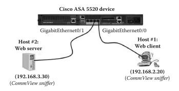
The following screenshot shows the configuration of GigabitEthernet0/0 (192.168.2.1/24) and GigabitEthernet0/1 (192.168.3.1/24) interfaces of the Cisco ASA 5520.
