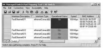
Once a packet is sent to one of these three victim hosts (Host #2, Host #3, or Host #4), the switch will forward it to Port #1, that is, to Host #1. This situation may create a DoS situation because the switch is not forwarding the packets, destined to these three hosts, to their legitimate destinations (see figure below).
