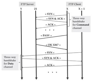
In addition, because FTP uses TCP-based channels, for each channel, four filtering rules are required to allow the corresponding traffic to pass through the firewall. For example, if the FTP client is an internal host and the FTP server is an external host, then the following table provides all the filtering rules for the Command and Data channels, respectively.
