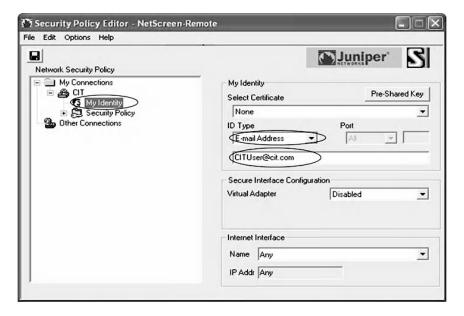
Next, click on the "Pre-shared Key" button, and then enter the key used in the VPN gateway configuration, which was "12345678", and click "OK" to complete the configuration as shown below.
