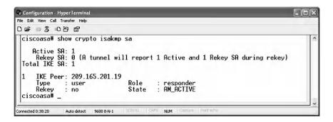
It is noticed that the number of active security associations is 1, the IKE peer is 209.165.201.19, the connection type is Remote Access VPN (user), the role of the remote user is responder, and the IKE phase 1 mode is aggressive as denoted by the "State : AM-ACTIVE." To display the IKE Phase 2 security association, type the following command: "show crypto ipsec sa".
