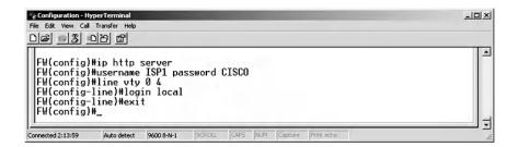
Configure the HTTP and Telnet servers on router BB1; repeat the steps followed for router FW.
