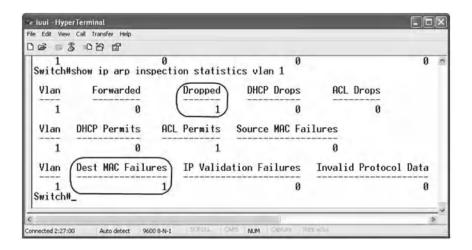
Packet #4: Host A sends the following abnormal ARP reply packet. The packet contains invalid destination IP address (255.255.255.255) in the ARP header, as shown below:
