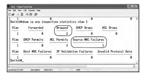
Packet #3: Host A sends the following abnormal ARP reply packet to Host B. The ARP packet has the destination MAC address in the Ethernet header different from the destination MAC address in the ARP header, as shown here:
