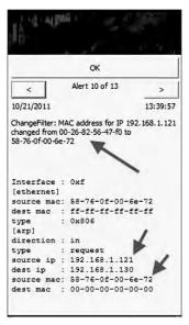
The XArp 2 ChangeFilter alert message indicates that the packet breaks current mappings. XArp 2 keeps track of IP-to-MAC address mappings. ARP requests contain the IP-MAC mapping of the sender. ARP replies contain the IP-MAC mapping of the host resolved. Every mapping is inserted into a database. If a monitored mapping breaks current mappings, an alert is generated.
