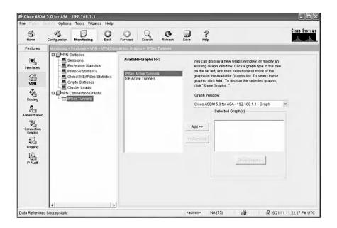
From the text area of available graphs, select "IPsec Active tunnel" and click the "Add" button to get the window shown below. Repeat the previous step with the IKE active tunnels, so that the IKE and IPsec active tunnels information will be shown in a graph.
