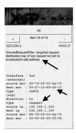
The XArp 2 DirectedRequestFilter alert message indicates that the ARP request packet is sent to a Unicast MAC address. However, ARP requests must be sent to the broadcast MAC address.
