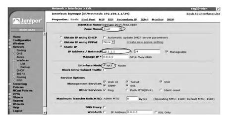
After changing the interface IP address, the Juniper WebUI automatically logs out. Therefore, change Al-Ain PC's IP address to 10.1.1.2/24, as shown below.
