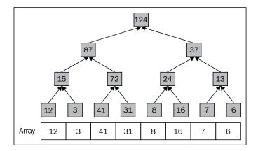
The previous diagram created juxtaposition, and it alters the way the same piece of data you saw, that is, one dimensional flat array containing arbitrary values. Imagine a tree of computations that scans and operates on two values. One way of storing those partial sums is to write the value in place to the array and another way is to use shared memory on the device.
