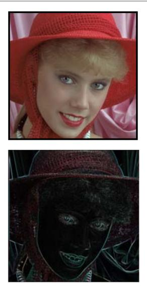
However, there is another nice optimization which we could have done, and it would have helped if we understood that a 3 X 3 convolution kernel (for example, the Sobel operator) is actually equivalent to the product of two vectors. This realization is behind the optimization algorithm also known as separable convolution.
