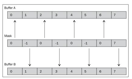
The following diagram illustrates this selection process. As before, once the selection process is completed, it is flushed out to the results vector, result.
