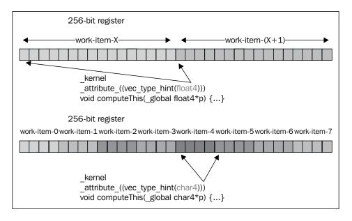
the compiler's implementation. The following figure is a conceptual view of how the OpenCL compiler might generate work items to consume the data in the wide registers:
