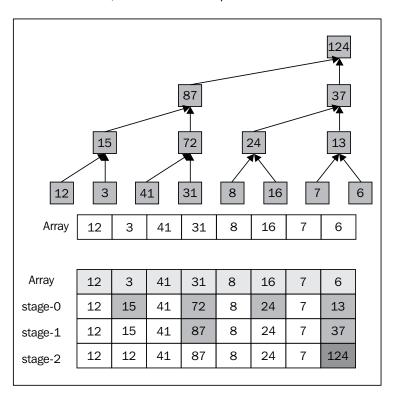
To be able to compute the prefix sums from the up-sweep phase we need to proceed from the root of this tree and perform a *down-sweep* using this algorithm by *Guy Blelloch*:
