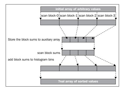
Let's look at how the block scan is done by examining blockScan. First, we load the values from the previously computed histogram bin into its shared memory as shown in the following code:
