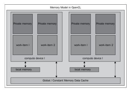
Applying the techniques we have learnt so far, we actually have one possible point in which we can apply shared memory techniques by looking out for code that is fetching data from the global memory. We will develop a solution using shared memory and expanding it slightly to have our program load it in strides. We'll get into that in a short while. Let's start at a plausible point for reworking our bitonicSort program taking into account the presence of shared memory:
