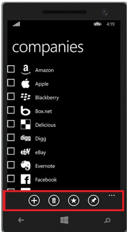
Figure 9-15. An Application Bar provides quick access to actions that can be performed on the current page
