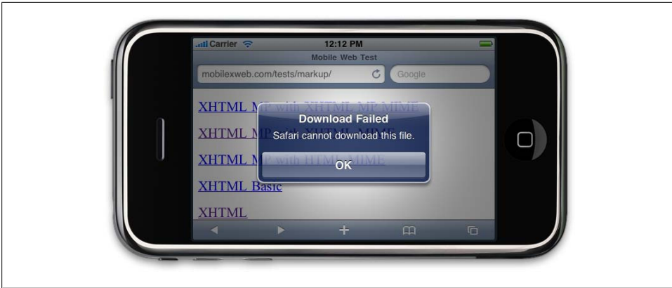
Figure 5-7. Safari on iOS doesn’t understand the XHTML MP MIME type, so documents for smartphones using this browser need to be served using non-mobile MIME headers.
