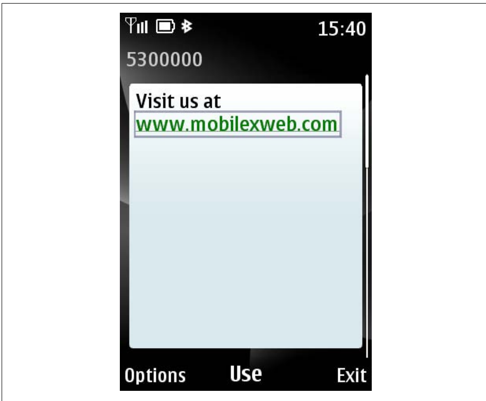
Figure 14-2. Modern devices detect URLs inside an inbound SMS and allow the user to access them with a click.
