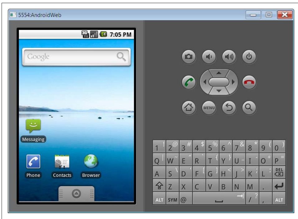
Figure 4-4. At this point, you can open the browser as if you were on a touch-enabled Android device. You can use the mouse over the emulator's screen to emulate the user's gestures.
