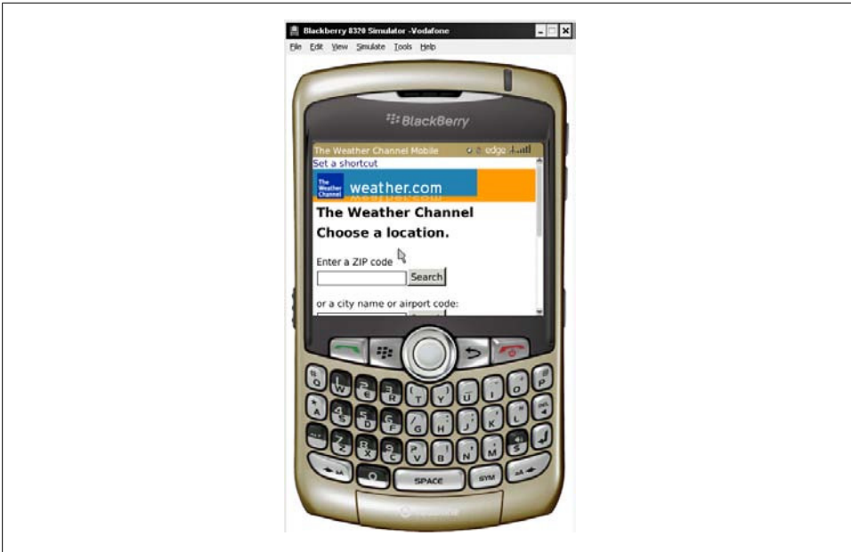
Figure 4-9. This BlackBerry simulator is pointer-based, so you need to use the onscreen keys or the arrow keys on your desktop keyboard to browse as a mobile user.
