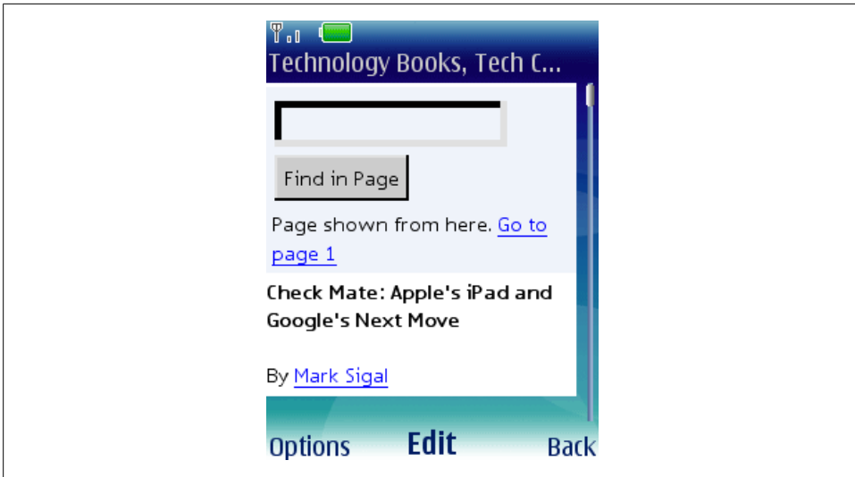
Figure 14-1. If you don't provide a mobile version of your website, Google will use its transcoder for users with low- or mid-end devices. Here is the O'Reilly home page transcoded.
