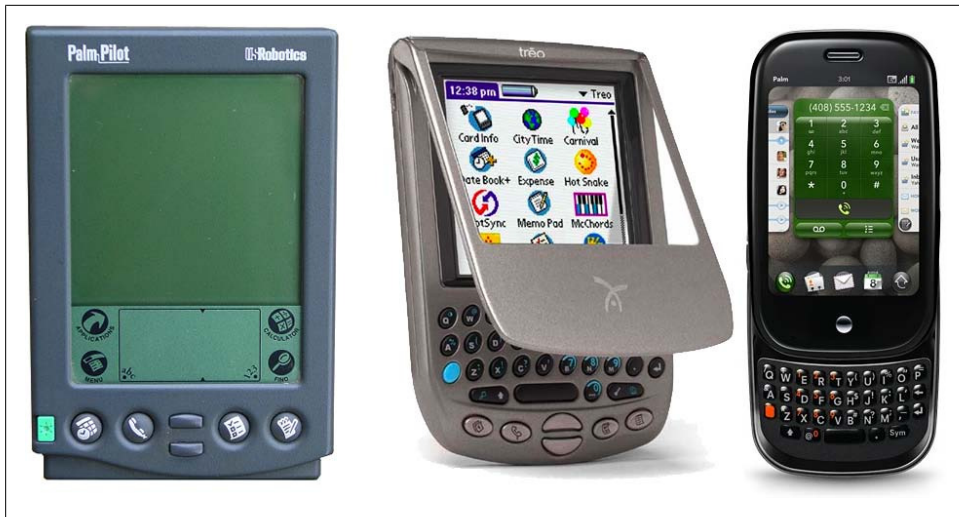
Figure 1-11. Palm has a really interesting history. Pictured here are the original USRobotics PalmPilot, the Handspring Treo, and the new webOS-based Palm Pre.
