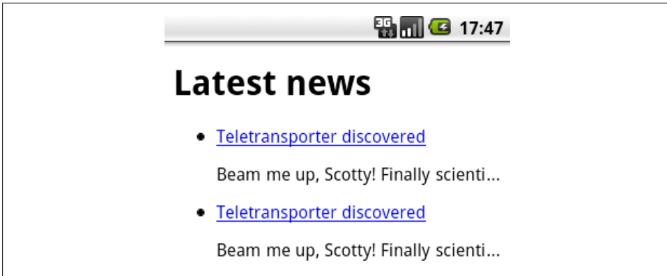
Figure 7-3. text-overflow: ellipsis is a great feature for displaying summaries in mobile designs.
