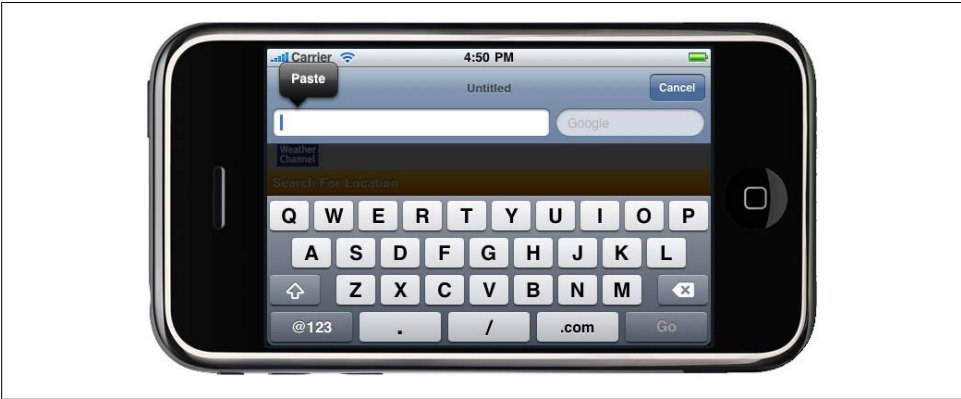
Figure 4-7. You can use your desktop keyboard, or Edit→Paste to paste text to the iPhone’s clipboard, and then tap once on the text input and press Paste on the screen to paste it where you want it to go.
