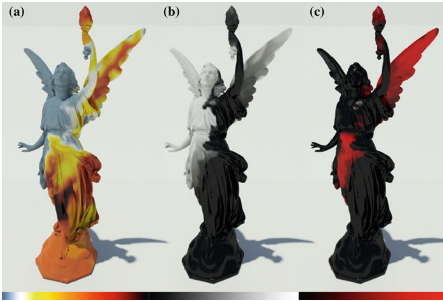
Fig. 4.15 Characteristics of a combustion waves: a temperature, b solid fuel remaining, c and reaction zones
