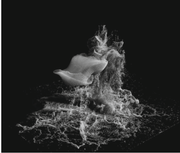
Fig. 5.6 Leaking particles in an SDF-based simulation
