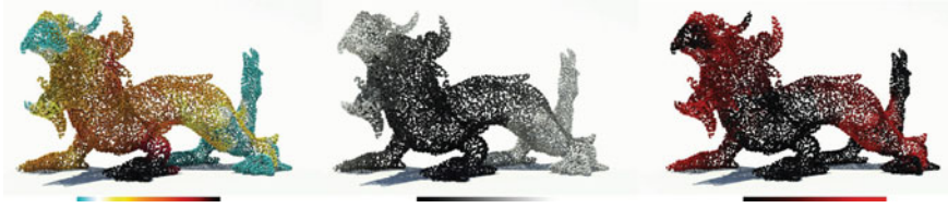
Fig. 4.13 Simulation of combustion waves on the surface of a point cloud: Heat transfer, fuel consumption, and reaction zones from the left . The heat transfer model includes diffusion and advection with airflow velocity fields to generate complicated flows
