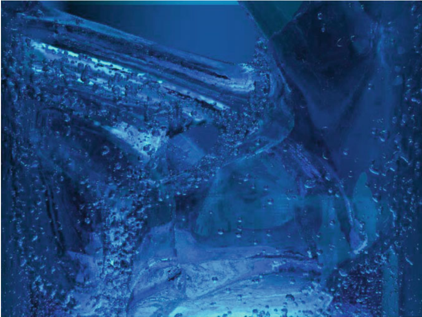
Fig. 5.16 Pouring water in an empty box generates numerous particles. Air bubbles on the right side of the figure are described in level set from merged particles
