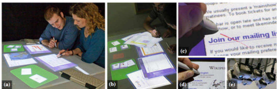
Figure 2.17: Websurface tabletop display. Users move and mark documents using styluses on the 6-projector high-resolution display. Source: [202]
