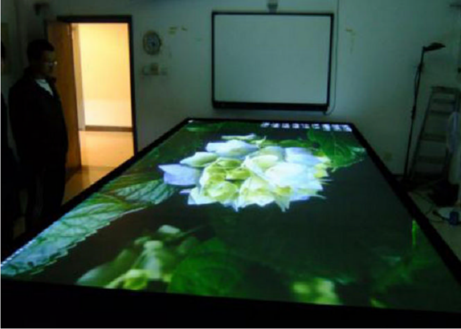
Figure 2.12: uMeeting: A tabletop display system. The uTable, which is part of the uMeeting system, is a rear-projected multi-touch display. Source: [124]
