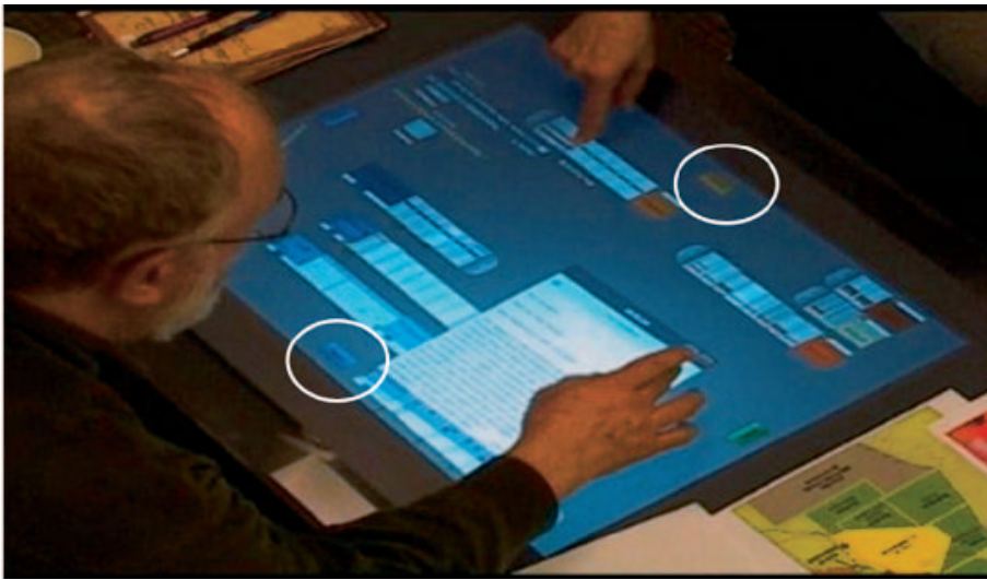
Figure 2.15: Touch-enabled tabletop to solve the 2006 VAST Challenge. Participants in the VAST challenge work together on a shared tabletop surface. Source: [93]
