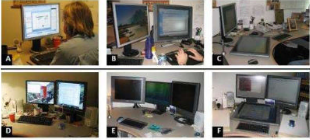
Figure 4.1: Testing the benefits of additional displays. Images a) and d) show two types of typical office environments: one display or two displays respectively. Images b) and e) show an additional vertical display inserted into the two types of environments. Images e) and f) show an additional horizontal display inserted into the two types of environments. Source: [137]
