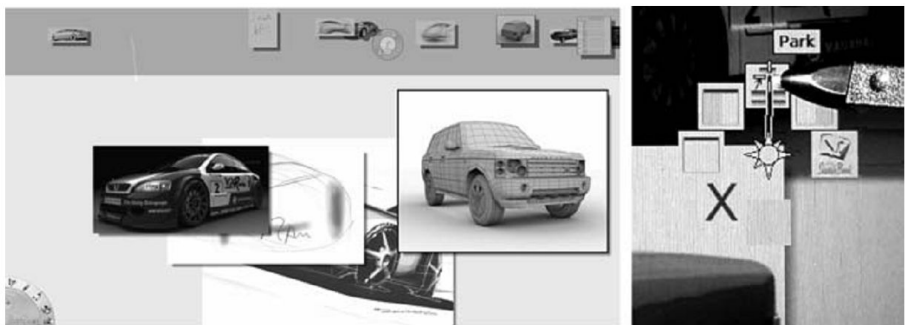
Figure 4.15: Sketchboard: An application designed for a large display for groups that collaborate with many artifacts. The large display shown on left displays four drawing artifacts in a central area and smaller icons of other artifacts in a strip at the top. To the right is a closeup of a TabletPC display view. Designers in the meeting interact with the large display using their TabletPC and a stylus. They can flick artifacts back and forth between the large display and their TabletPC. Both displays show specially designed circular interaction menus. Source: [106]
