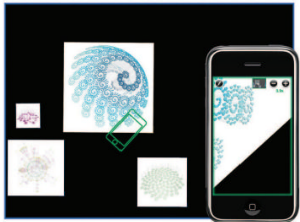
Figure 3.1: Selecting high resolution items with a low resolution pointing device. A solution to the ‘fat fingers’ problem encountered when using tabletop displays. A smartphone displays an enlarged image of a part of the tabletop display. The user selects a part of the image by touching the smartphone display. Source: [211]
