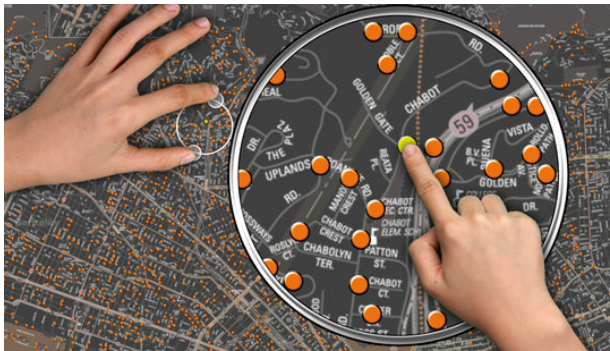
Figure 3.2: FingerGlass: A widget for interacting with large displays. The FingerGlass widget helps users see more detail and helps with precise selection. Source: [104]
