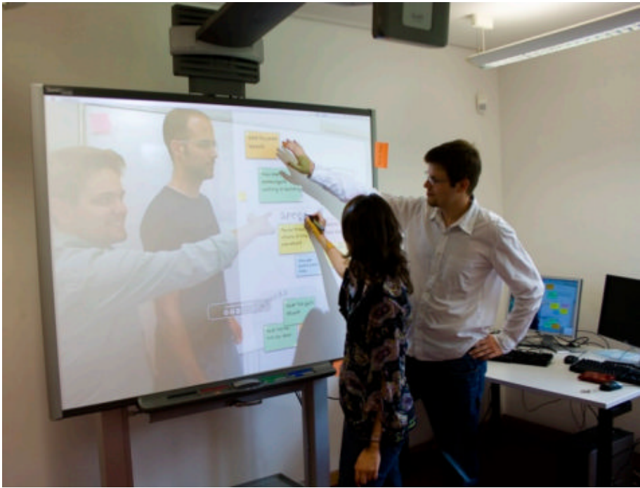
Figure 2.13: Teleboard display system. Creative designers collaborate over long distance using a mixture of touch and pen gestures on a projected whiteboard. Source: [74]
