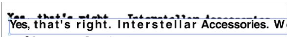
Figure 42: This text imprint was derived from an OCR analysis of a low-resolution JPEG image that was scanned from a decades-old typed letter. Note the default font, Helvetica 12, was used in the imprint, and that the imprint does not quite align with the underlying text image, which was scanned at a slight angle.
