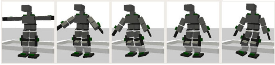
Fig. 8. Time series of the robot controlled by a resulting network for the march-in-place task.
