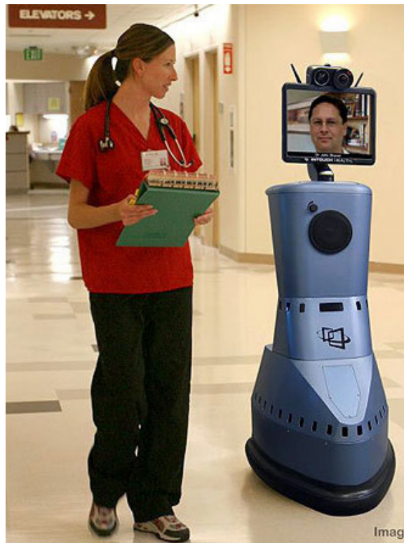
Figure 2.7: The InTouch Health telemedicine robot, with video conferencing on a remote controlled unit. Copyright © 2013 InTouch Technologies, Inc. Used with permission.
