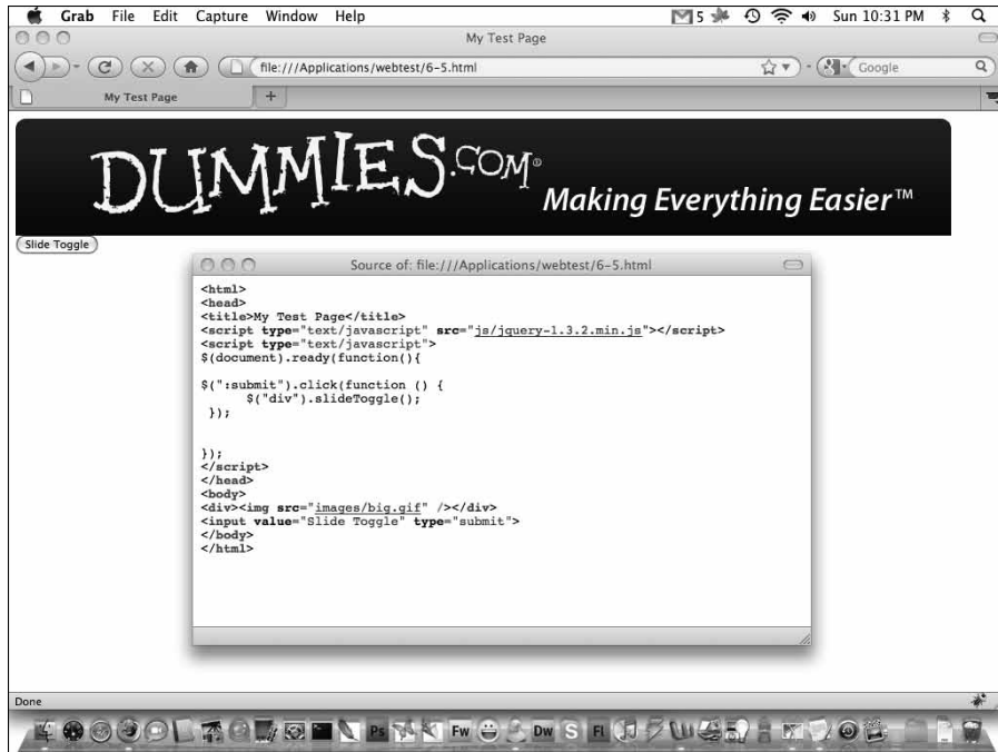
Figure 6-5: When you click the button, the <div> element toggles between sliding up and down.
