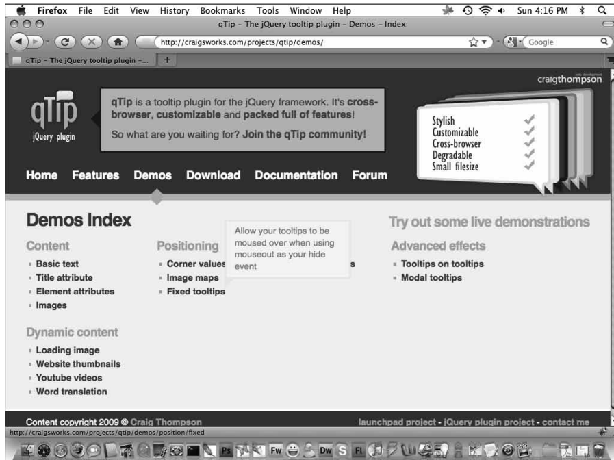
Figure 20-3: A tooltip window appears when a link is moused over with the qTip plug-in.
