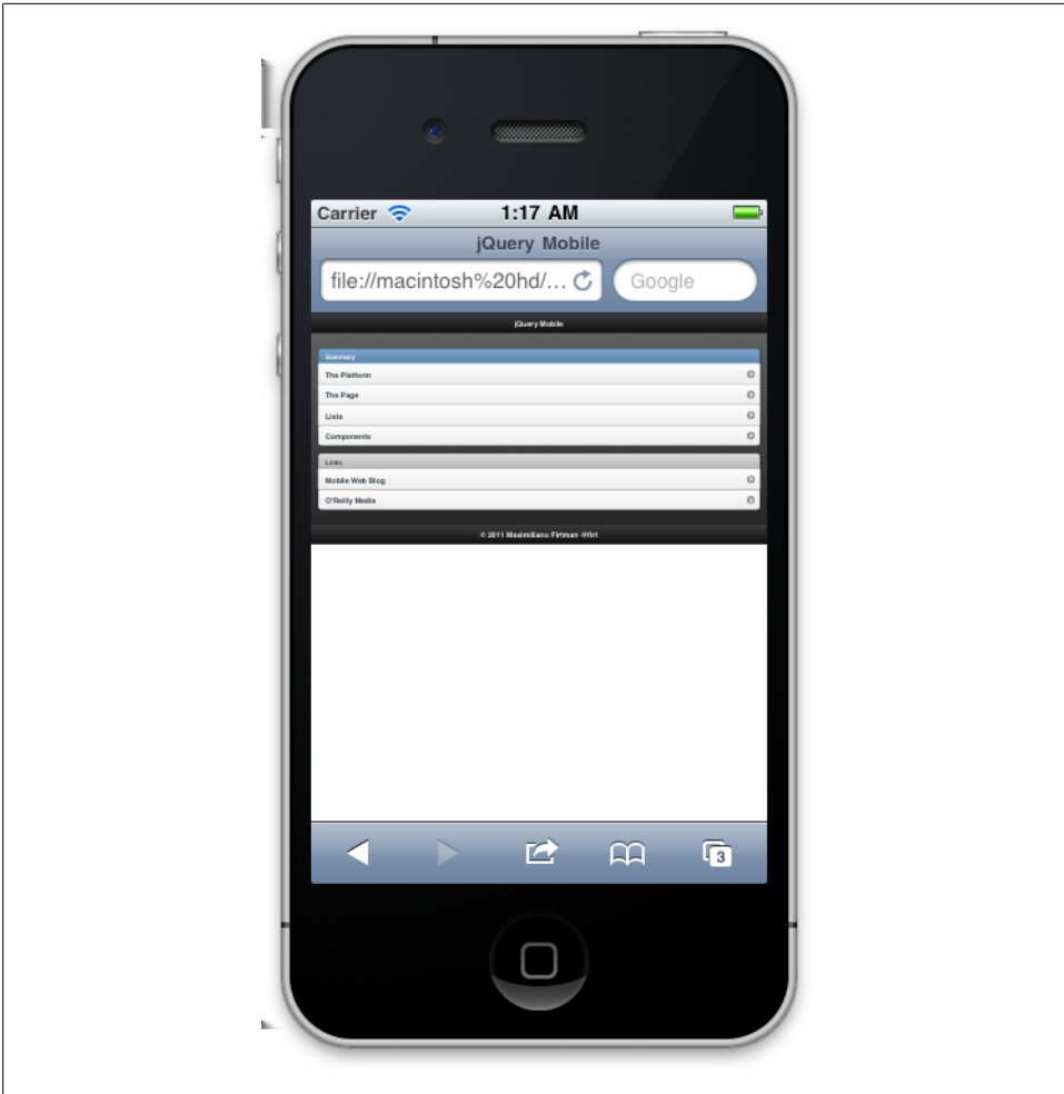
Figure 2-1. In jQuery Mobile we need to define a viewport meta tag to avoid this kind of UI problems when loading our webapp
