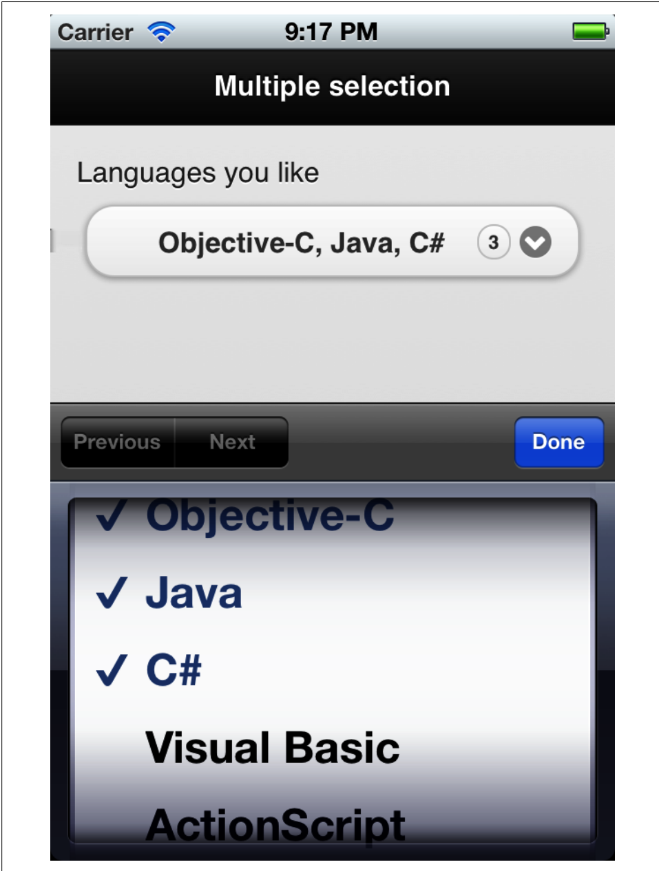
Figure 5-9. When using a multiple selection menu, the user interface shows us the selected elements separated by a comma and a count bubble showing how many elements were selected
