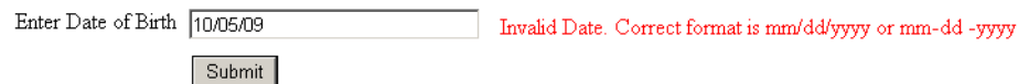
Figure 4-11. Error message: Invalid Date is displayed if the date is entered incorrectly.
