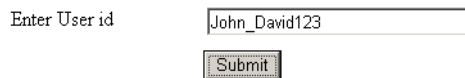
Figure 4-10. The user ID is considered valid if it consists of characters, numerals, and the underscore symbol.
