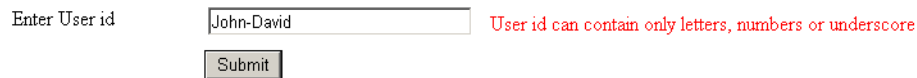
Figure 4-9. Error message displayed if any symbol other than the underscore is used in the user ID
