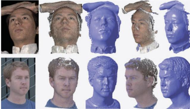
**Figure 1.7** Sample results on 3D modeling algorithm for calibrated multiview stereopsis proposed by Furukawa and Ponce (2010) that outputs a quasi-dense set of rectangular patches covering the surfaces visible in the input images. In each case, one of the input images is shown on the left, along with two views of textured-mapped reconstructed patches and shaded polygonal surfaces. Copyright © 2007, IEEE
