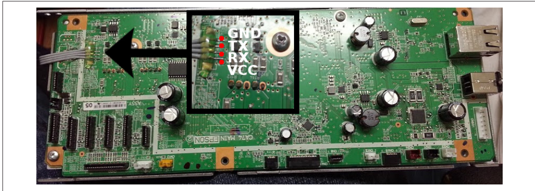
FIGURE 7-26. UART communication pins
