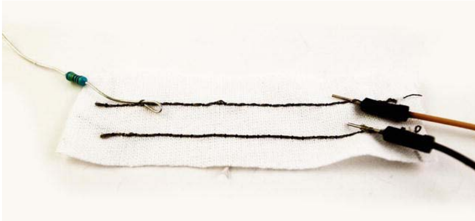
Figure 9-7. Making a test sensor
