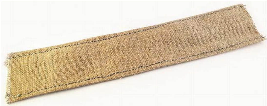
Figure 5-12. Seams sewn with conductive thread
