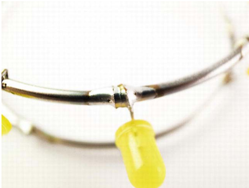
Figure 5-24. The solder should spread onto the material.
