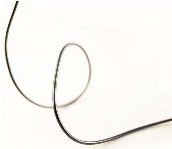
Figure 4-9. Smart wire that remembers shapes
