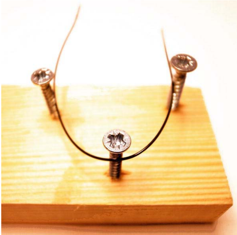
Figure 12-12. Reprogramming the SMA wire
