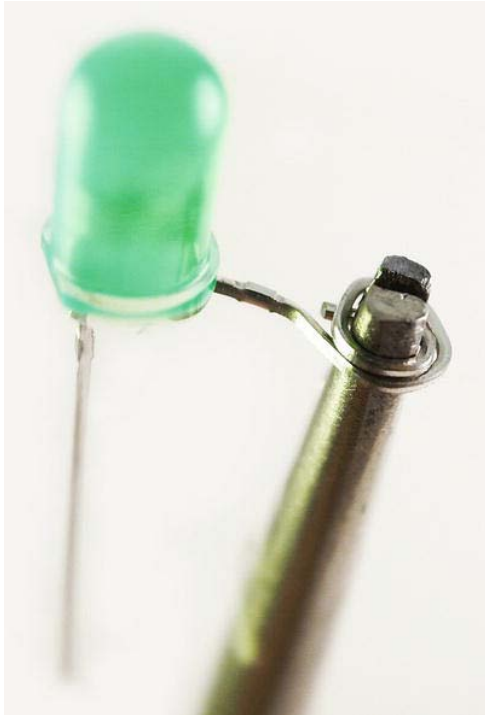
Figure 5-13. Modifying the LED legs
