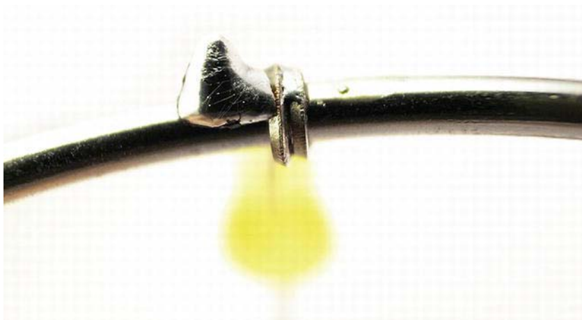
Figure 5-23. A cold soldering joint
