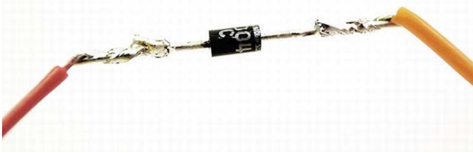
Figure 6-3. Diode connected between the solar panel and battery
