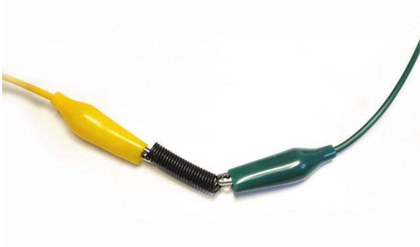
Figure 12-2. The SMA wire when it has reached the original position
