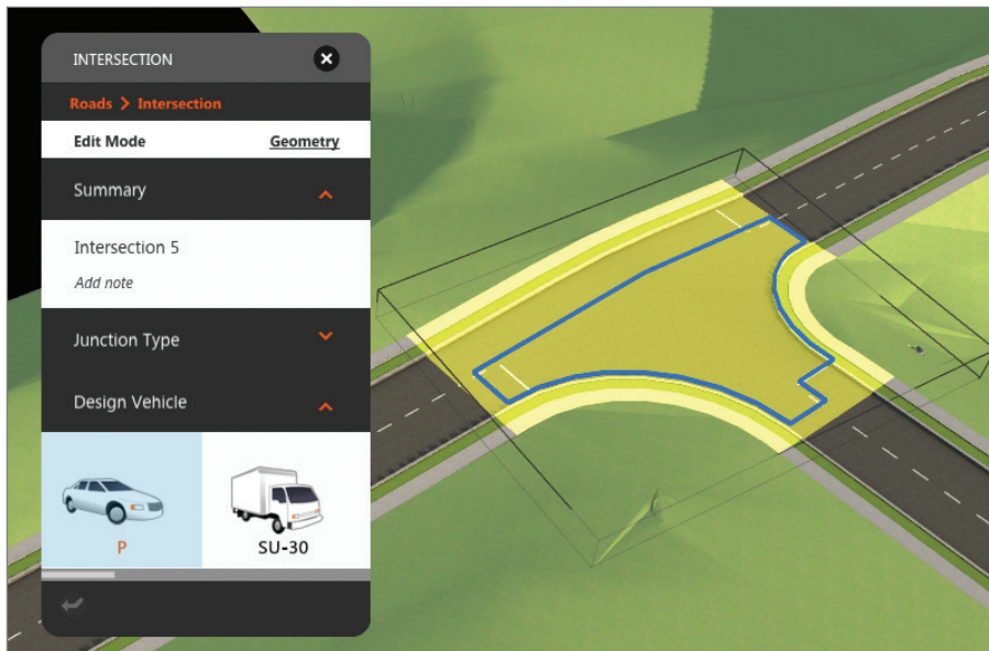
FIGURE 1.4 A specialized asset card for intersections
