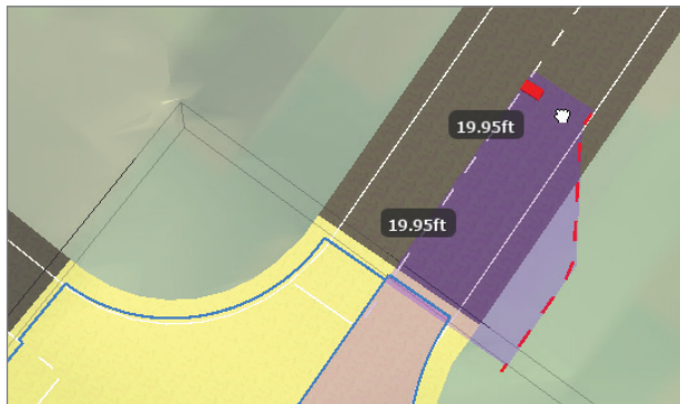
FIGURE 2.39 The purple cylinder gizmo (shown in red because it is selected) is used to add a widening zone.
