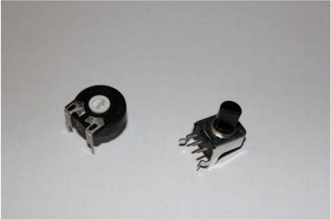
Figure 4-12. Potentiometer: trimmer (left), rotary potentiometer (right)
